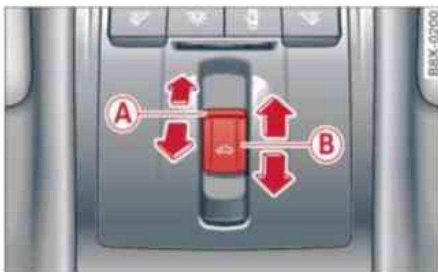
Fig. 49: Detail of headliner: Button for panorama sun roof
