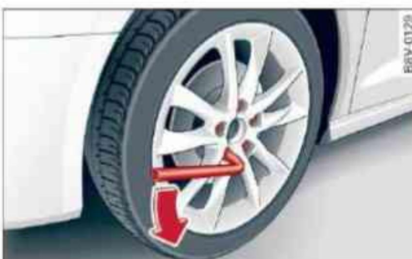
Fig. 242 Wheel: Loosening the wheel bolts
