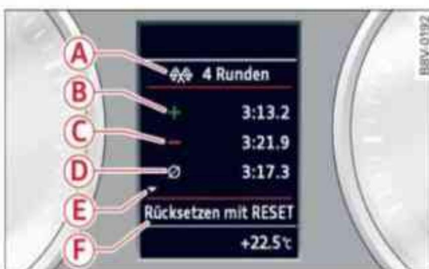
Fig. 29 Instrument cluster: Evaluating lap times
