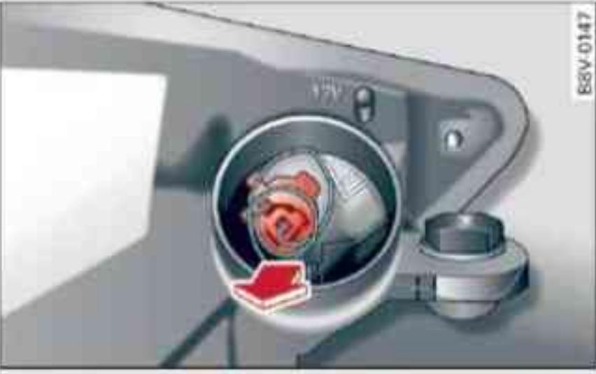
Fig. 279 Bulb holder for turn signal
