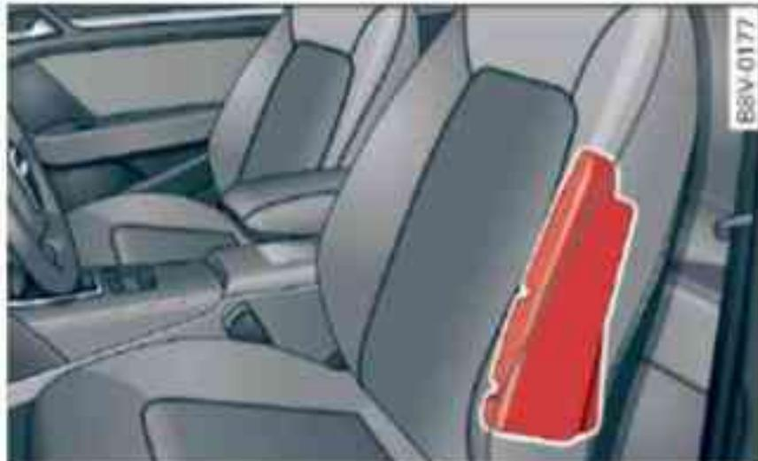
Fig. 194 Side airbags: Location in driver's seat (example)
