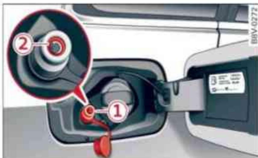
Fig. 116 Tank flap open: Gas filter neck (1) and filter neck seal (2)
