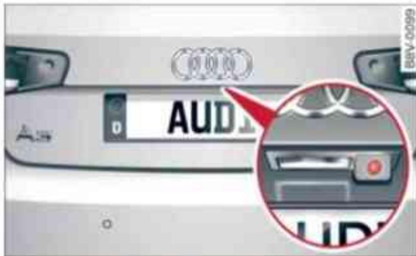
Fig. 153 Boot lid: Location of reversing camera (example)
