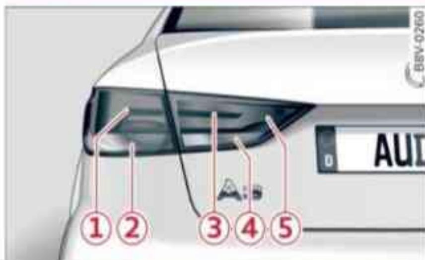
Fig. 266 Halogen system, rear light: Bulbs in side panel and boot lid
