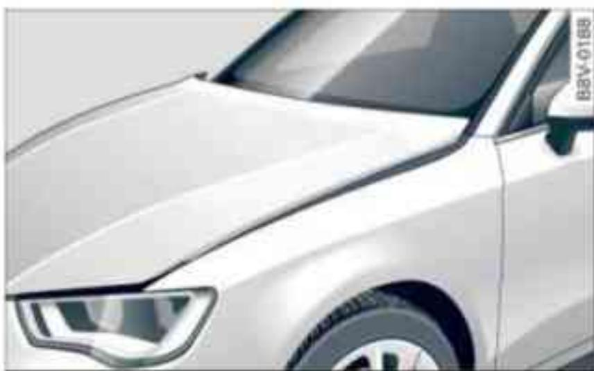
Fig. 174 Bonnet: Pedestrian protection system triggered
