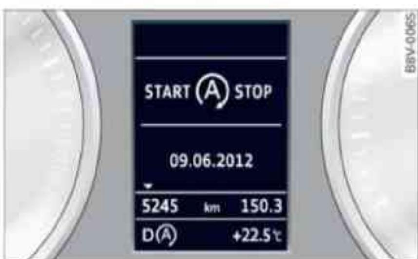
Fig. 109 Instrument cluster: Engine switched off (stop phase)
