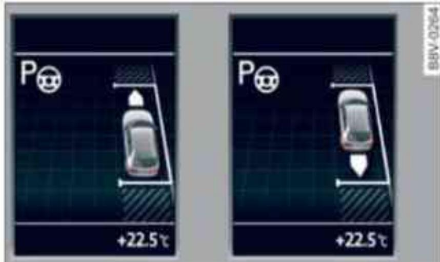
Fig. 165 Instrument cluster: Manoeuvring several times in a parking space
