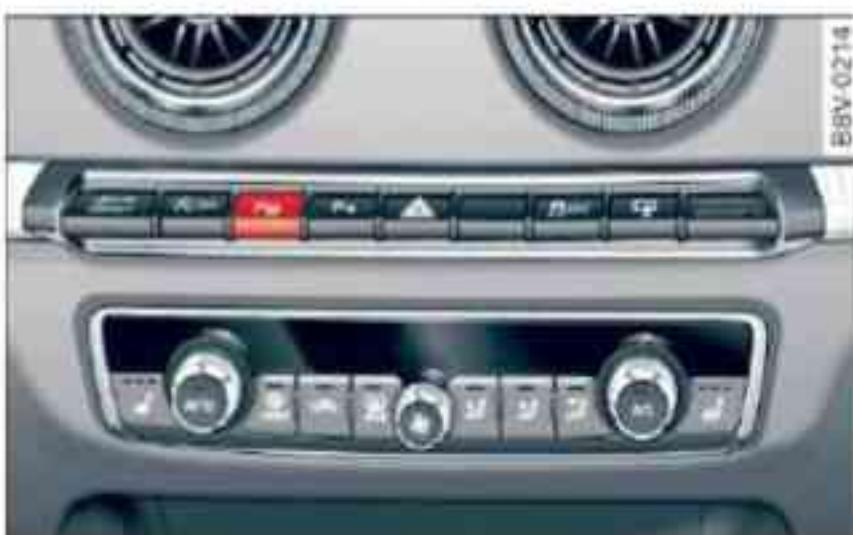
Fig. 161 Centre console: Switch for park assist
