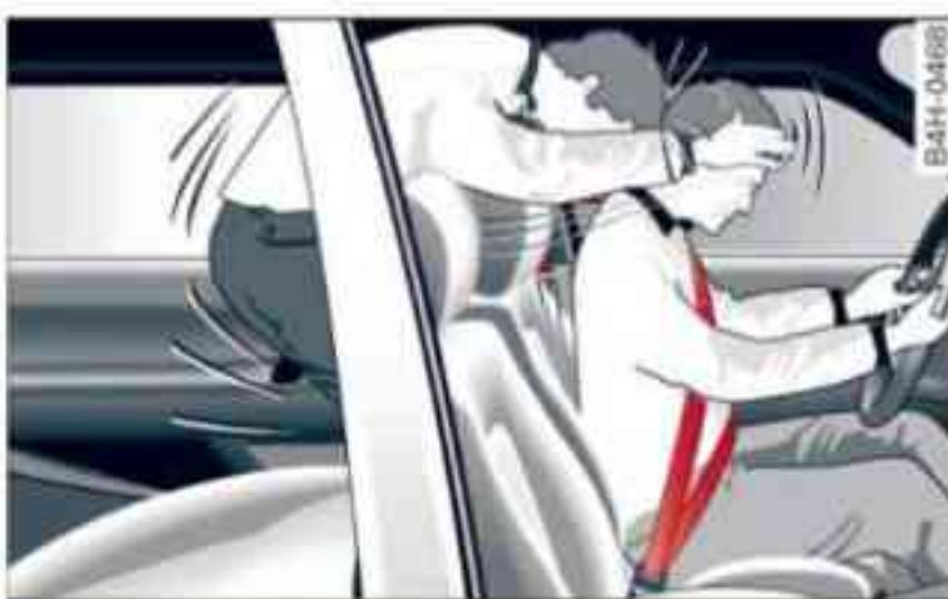
Fig. 180 A rear passenger not wearing a seat belt can be thrown forwards
