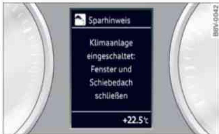
Fig. 22 Instrument cluster: Economy tip (Air conditioner switched on: close windows and sun roof)
