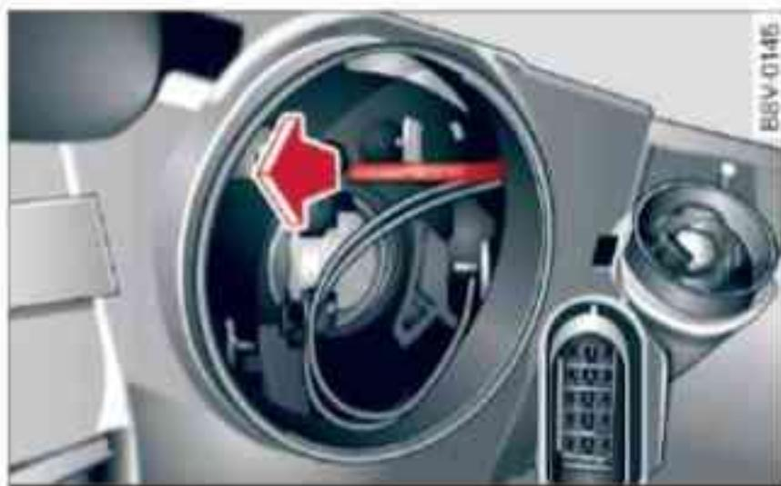
Fig. 276 Bulb holder for side lights
