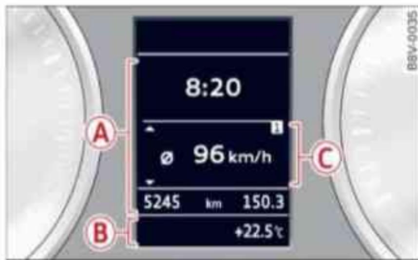
Fig. 12 Instrument cluster: Driver information system
