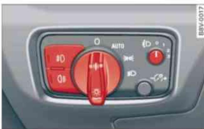
Fig. 50 Dashboard: Light switch with headlight range control
