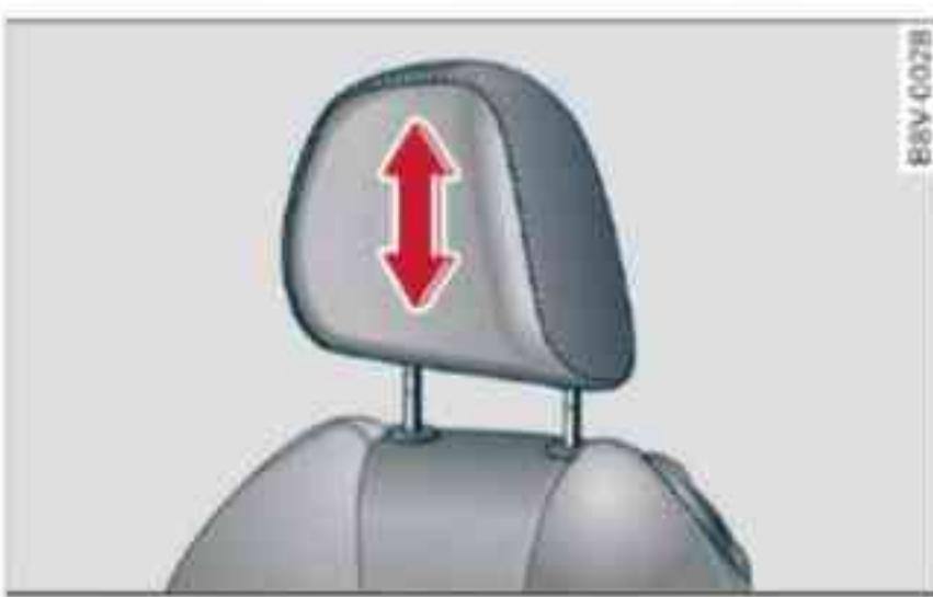
Fig. 72 Front seat: Adjusting standard head restraint
