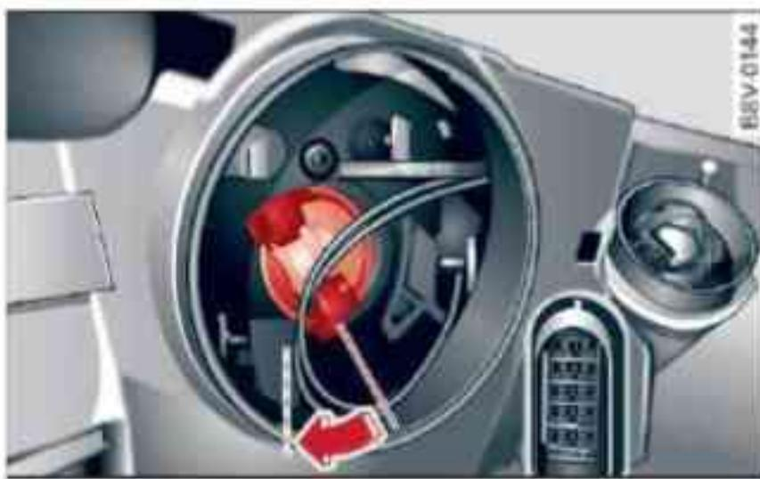
Fig. 274 Bulb housing: Fitting the bulb
