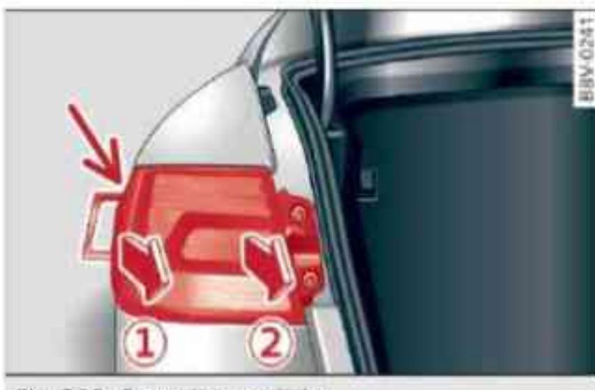
Fig. 308 Removing rear light
