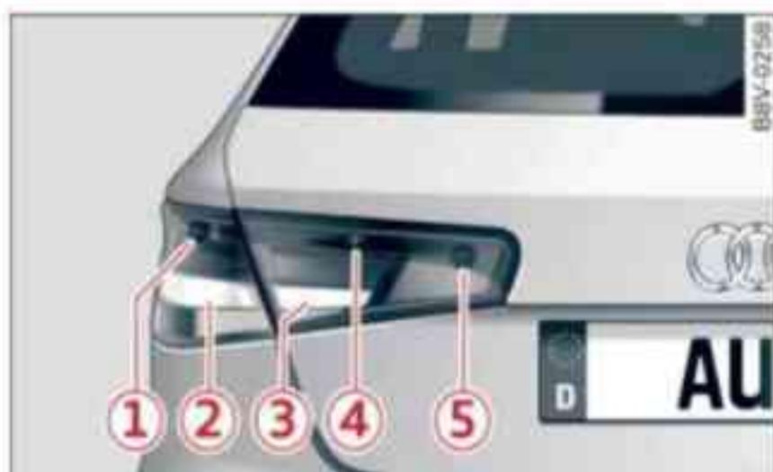
Fig. 262 Halogen system, rear light: Bulbs in side panel and boot lid
