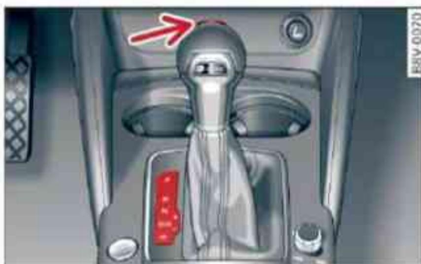
Fig. 119 Detail of the centre console: Selector lever with interlock button
