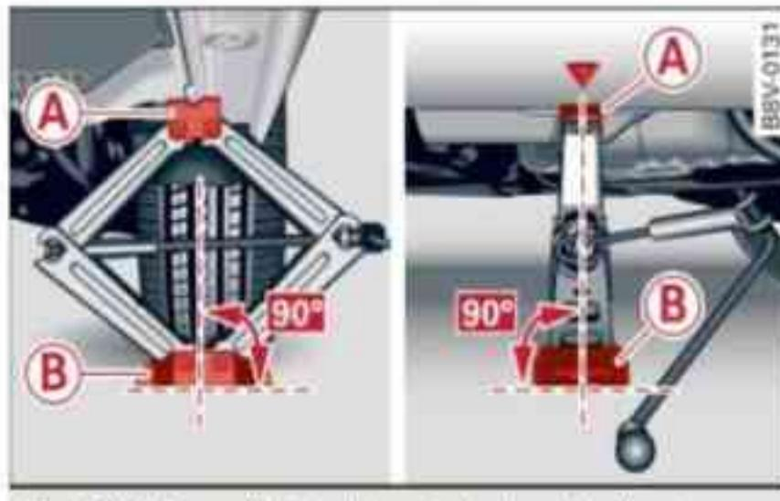
Fig. 244 Door sill: Applying the jack under the door sill
