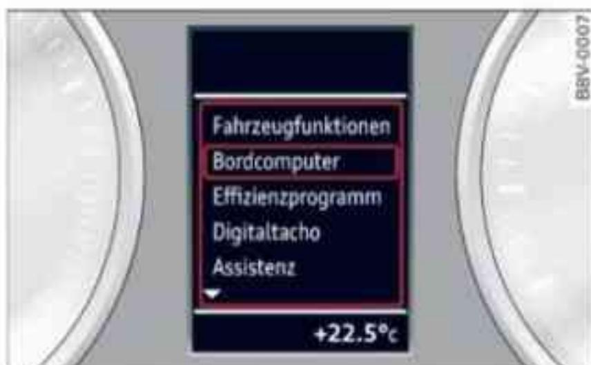
Fig. 16 Driver information system: Calling up the Vehicle functions menu
