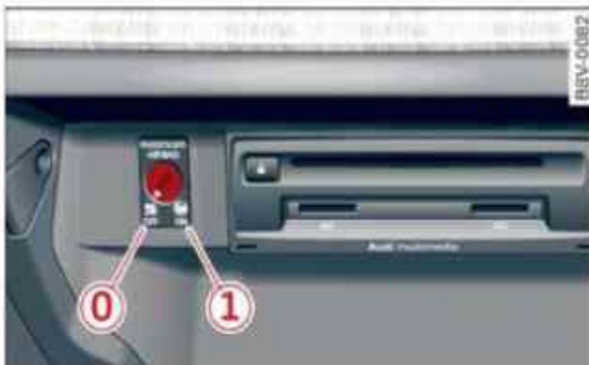
Fig. 198 Glove box: Key-operated switch for deactivating front passenger's airbag
