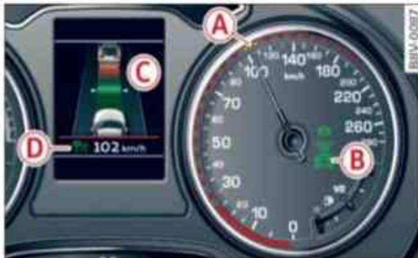
Fig. 131 Instrument cluster display: adaptive cruise control
