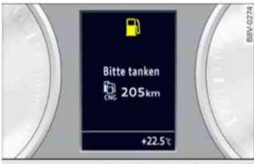
Fig. 114 Display: Combined fuel warning for petrol and natural gas
