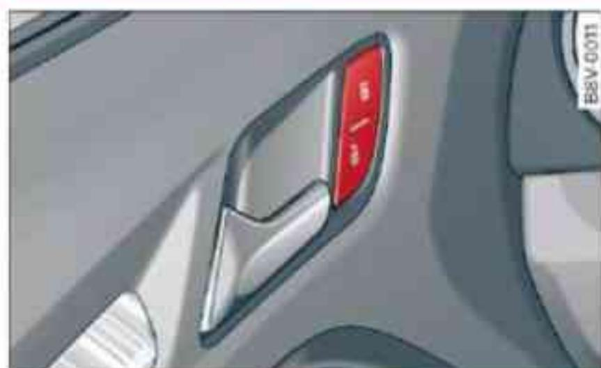
Fig. 39 Driver's door: Central locking switch
