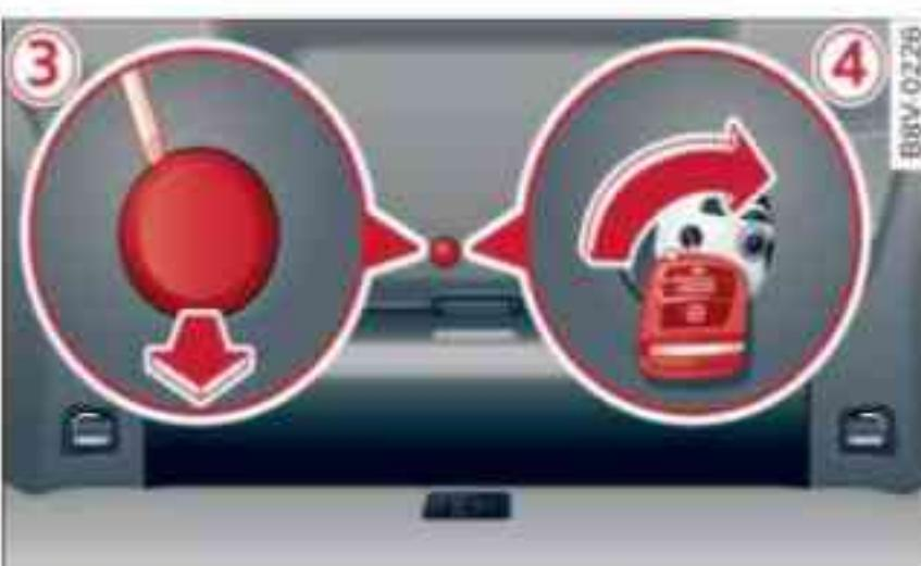
Fig. 45 (A3/A3 Saloon) Detail of inside of boot lid: Access to manual release
