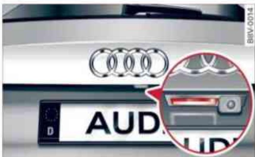
Fig. 42 Boot lid: Opening (release catch)
