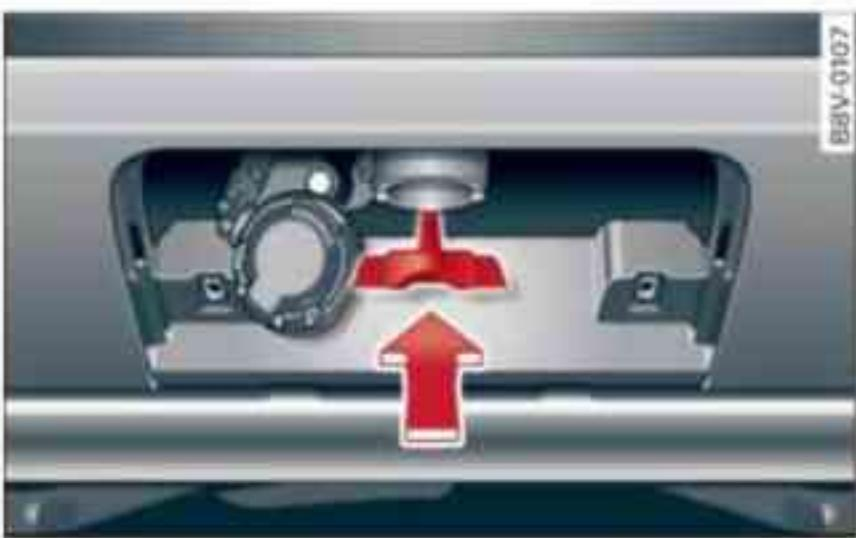
Fig. 211 Area below rear bumper: Fitting the plug
