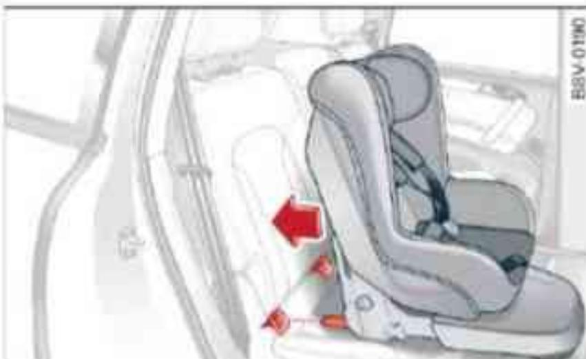
Fig. 170 Rear seat: Securing child seat with ISOFIX (example)
