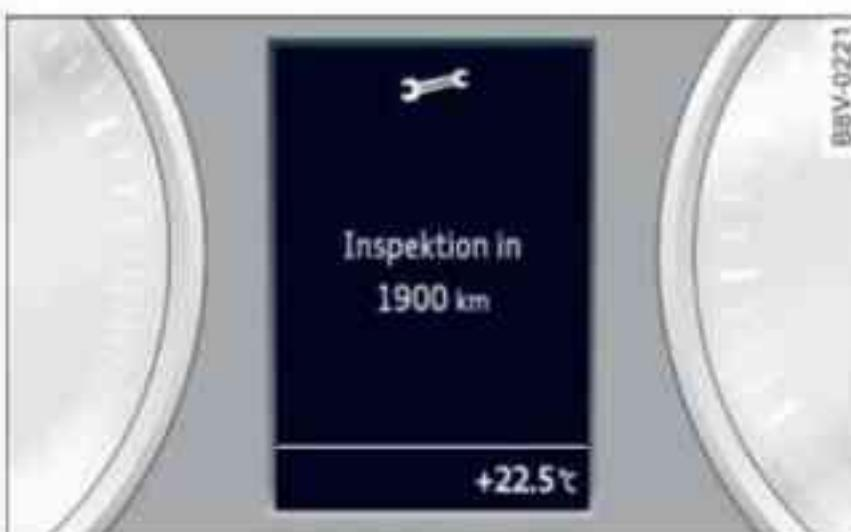
Fig. 9 Instrument cluster: Service interval display (example)
