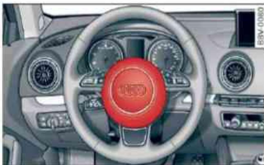
Fig. 188 Steering wheel: Driver's airbag
