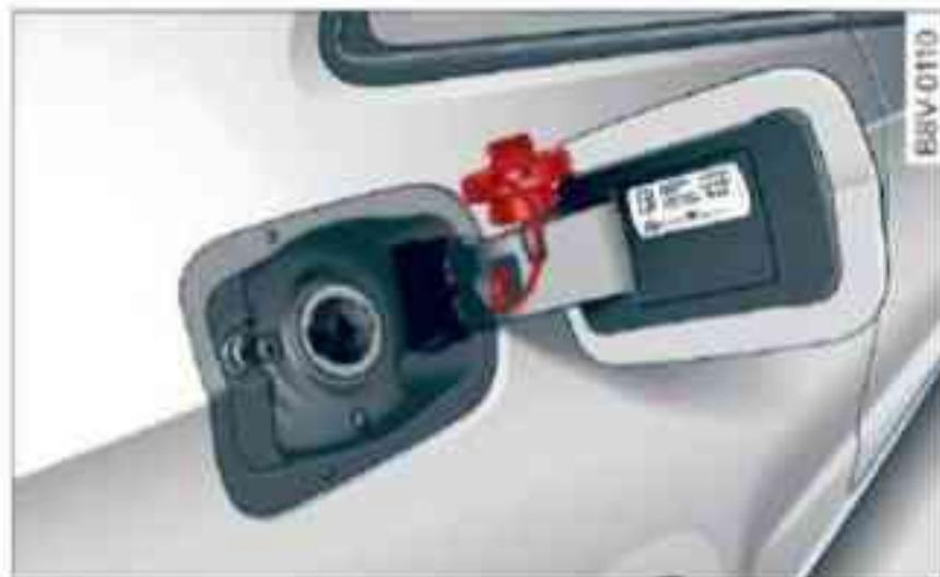
Fig. 216 Fuel tank flap with tank cap attached
