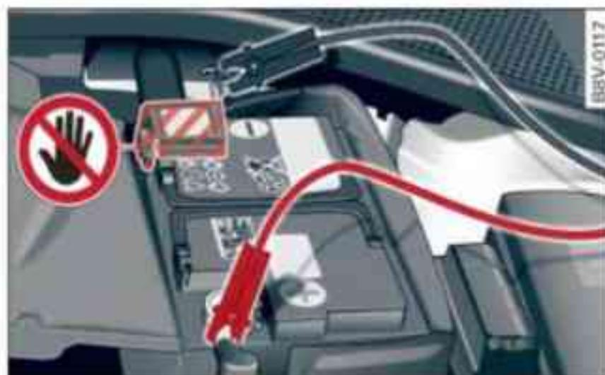
Fig. 225 Engine compartment: Terminals for jump leads and battery charger
