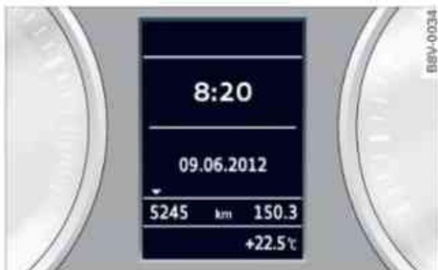
Fig. 6 Instrument cluster: Display without driver information system
