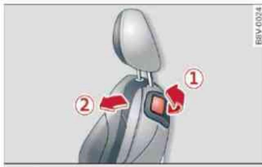
Fig. 68 Driver's seat: Easy entry controls
