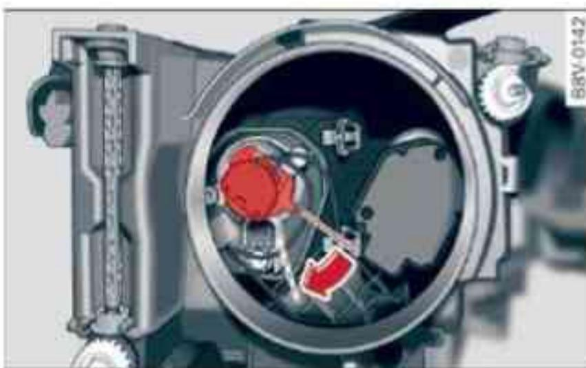
Fig. 271 Bulb housing: Fitting the bulb
