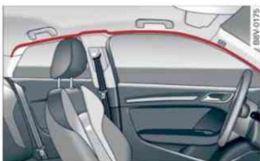
Fig. 196 Location of head-protection airbags above the doors (example)
