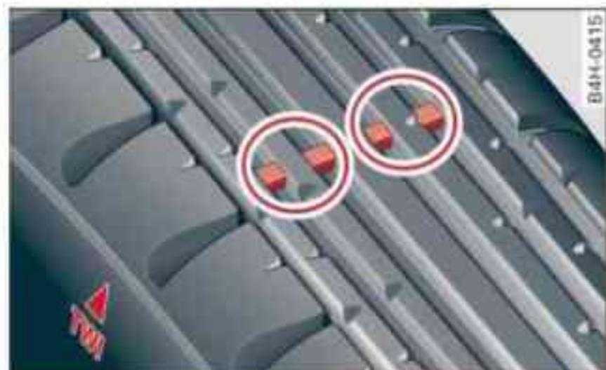
Fig. 228 Tyre tread: Tread wear indicators
