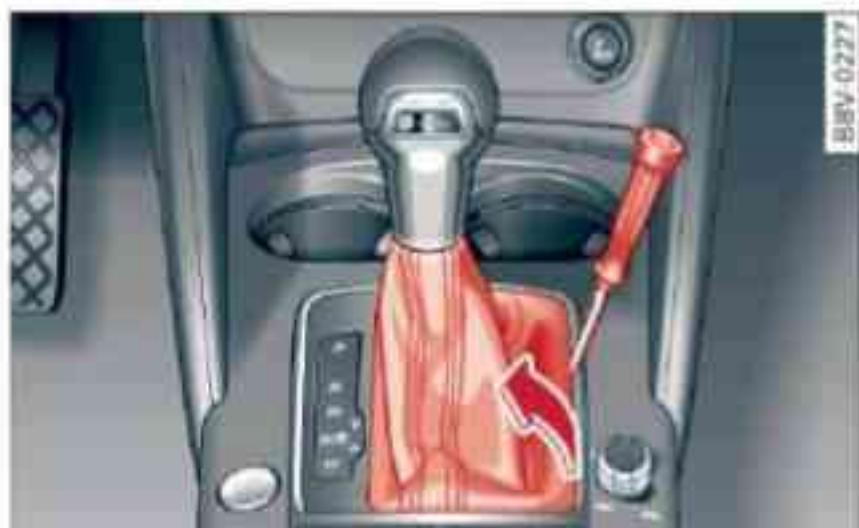
Fig. 122 Selector lever: Removing the cover
