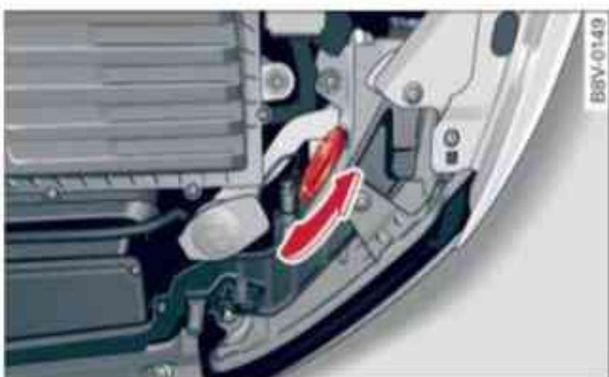
Fig. 284 Engine compartment: Removing cover on bulb housing
