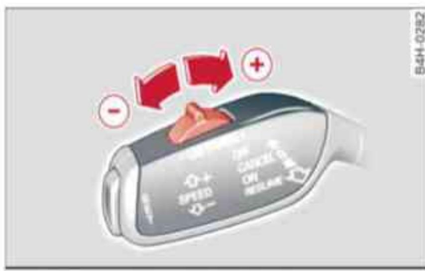
Fig. 134 Control lever: Setting the distance
