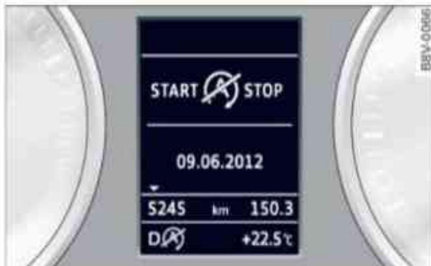
Fig. 110 Instrument cluster with driver information system: Engine stop temporarily unavailable
