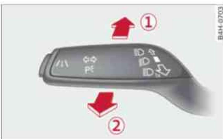
Fig. 54 Turn signal and main beam lever: Switching adaptive headlight range control on/off
