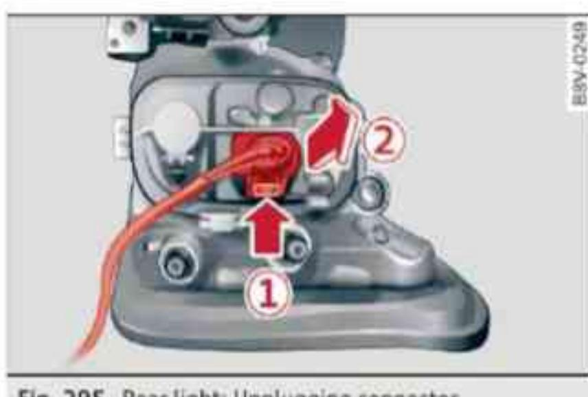
Fig. 295 Rear light: Unplugging connector
