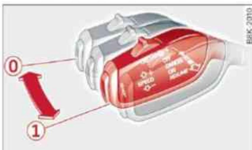
Fig. 130 Control lever: Switching on/off
