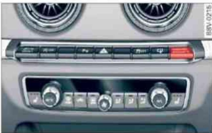
Fig. 199 Centre console: Warning lamp lights up when passenger's airbag is deactivated
