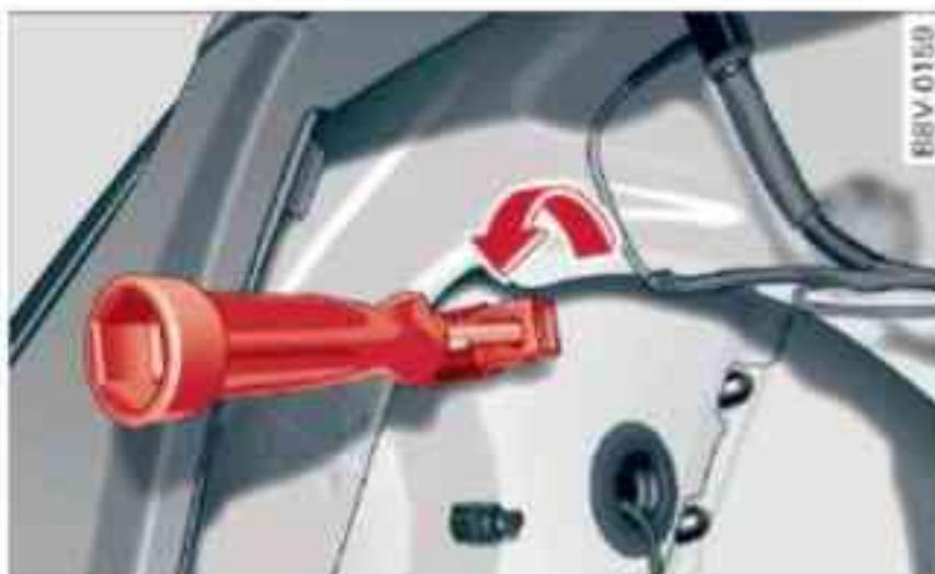
Fig. 291 Releasing rear light from luggage compartment (example on left side)
