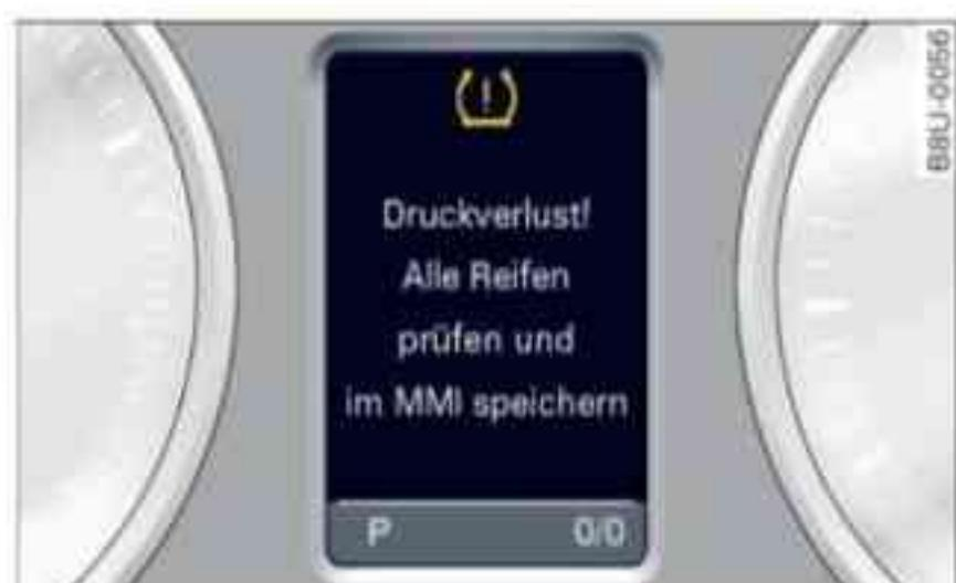
Fig. 230 Instrument cluster: Indicator lamp with message
