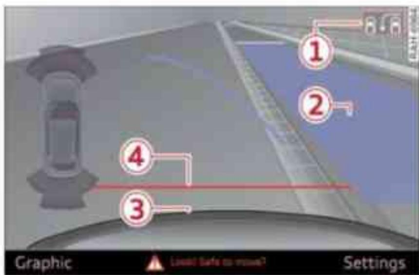
Fig. 156 MMI: Blue area marking aligned in parking space
