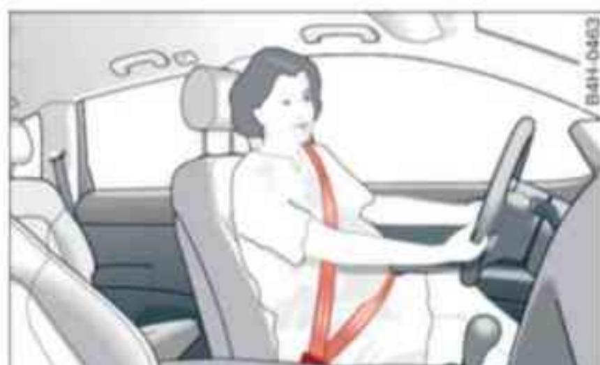
Fig. 184 Positioning seat belts during pregnancy
