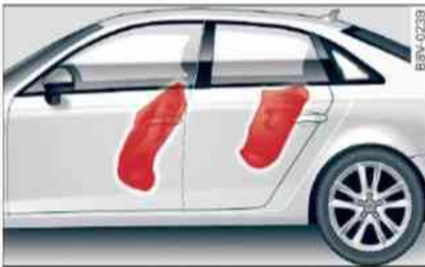
Fig. 195 Inflated front and rear\* side airbags (example)
