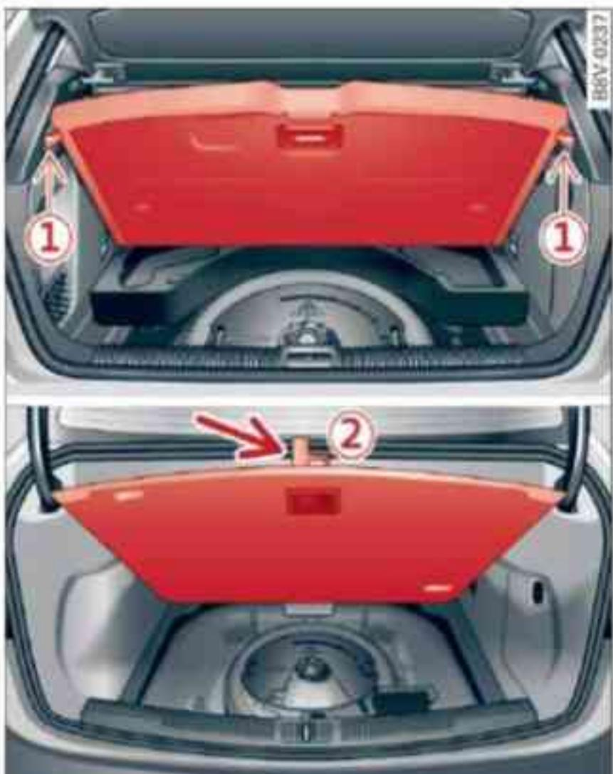
Fig. 236 Luggage compartment: Floor panel folded up (A3 and A3 Sportback top, A3 Saloon bottom)
