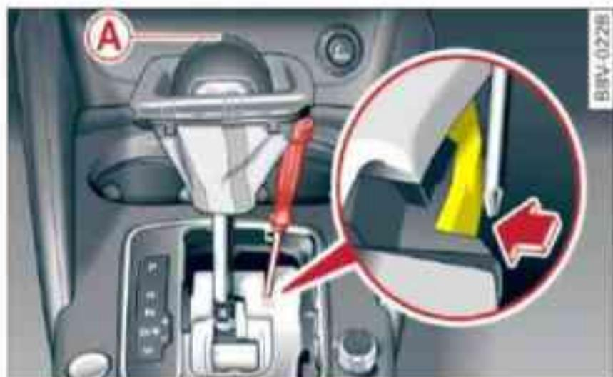
Fig. 123 Manually releasing the selector lever from position P
