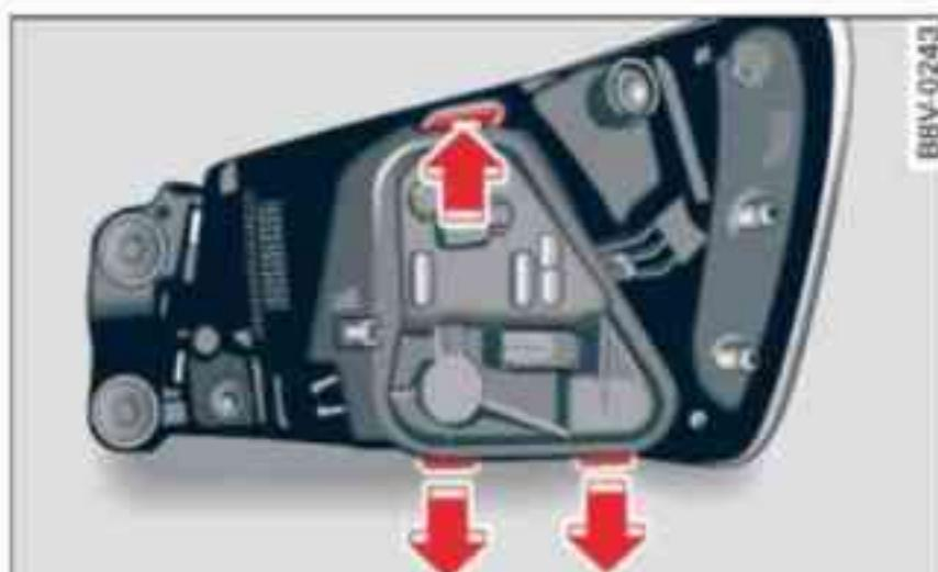
Fig. 310 Securing tabs between bulb carrier and rear light
