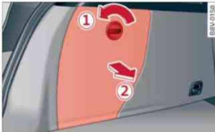
Fig. 290 Luggage compartment: Location of the retaining screw for the rear light (example on left side)
