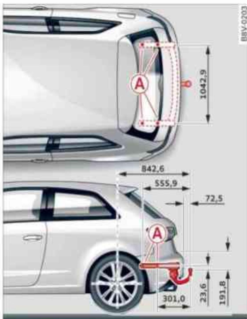
Fig. 212 A3: Positions of securing points (viewed from above and from side)
