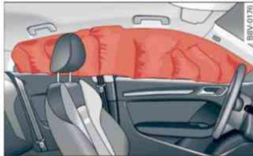
Fig. 197 Head-protection airbags in inflated condition (example)
