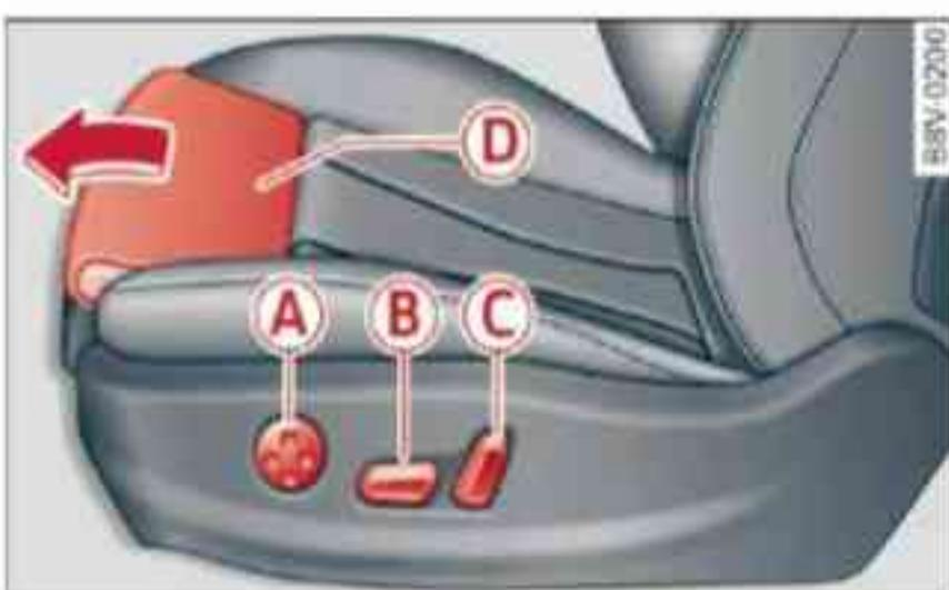
Fig. 67 Front seat: Electric adjustment
