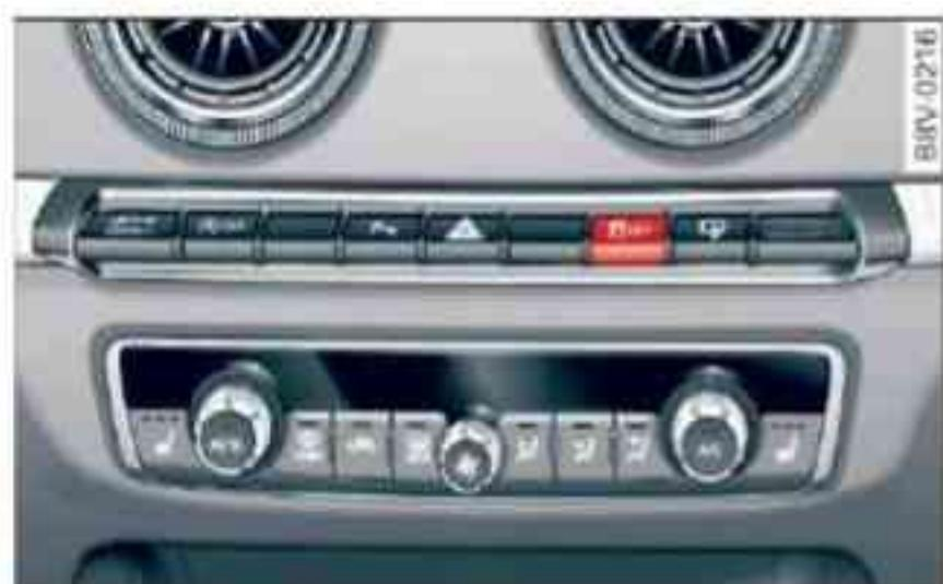
Fig. 200 Centre console (top): ESC button
