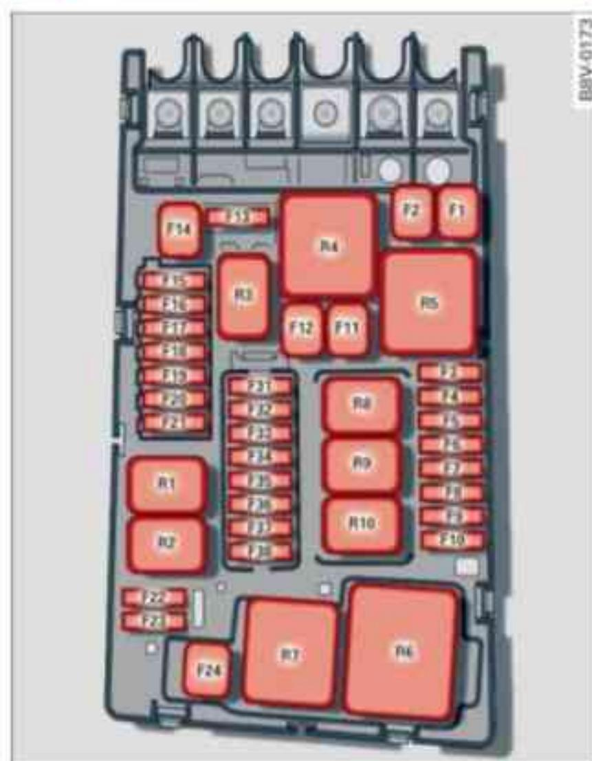
Fig. 259 Engine compartment: Fuse layout
