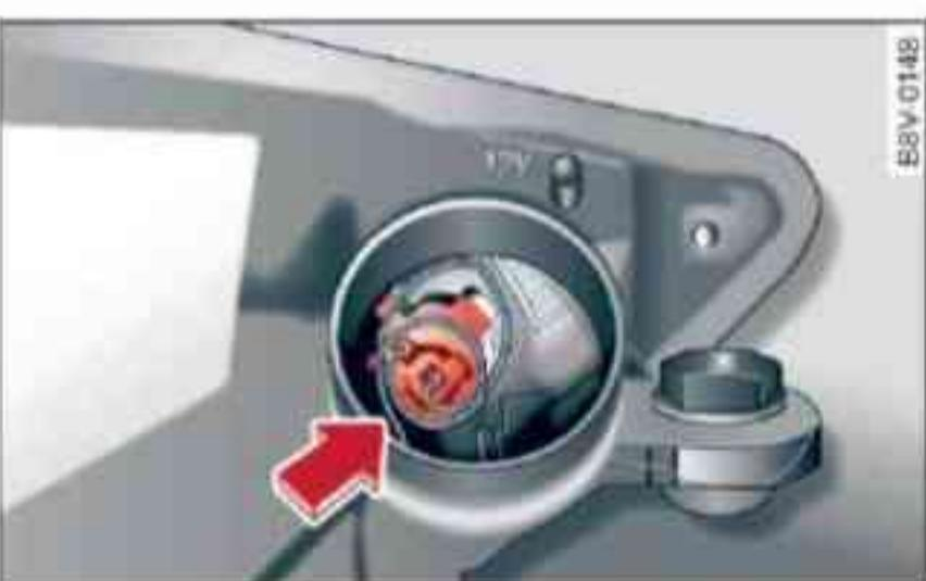
Fig. 280 Bulb housing: Inserting the bulb holder
