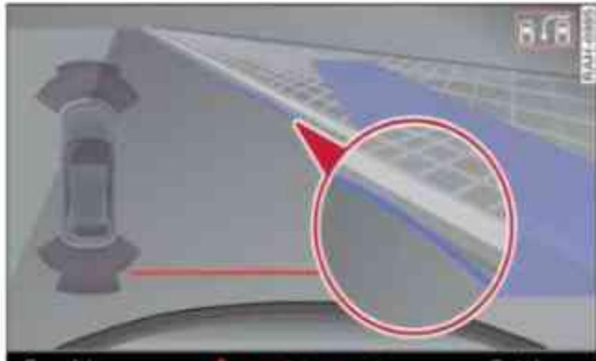
Fig. 157 MMI: Blue marking touches edge of pavement
