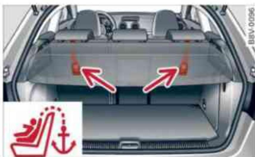
Fig. 171 Rear seat bench (A3/A3 Sportback): Top tether anchorages
