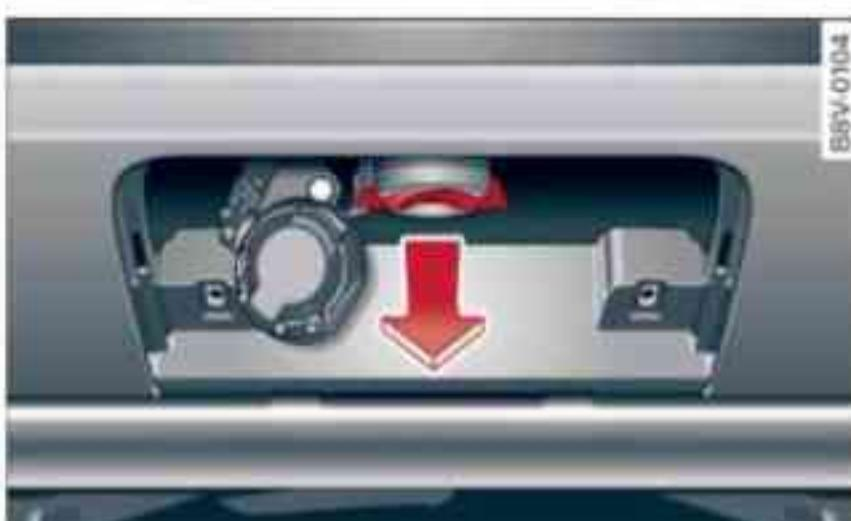
Fig. 204 Area below rear bumper: Pulling out plug
