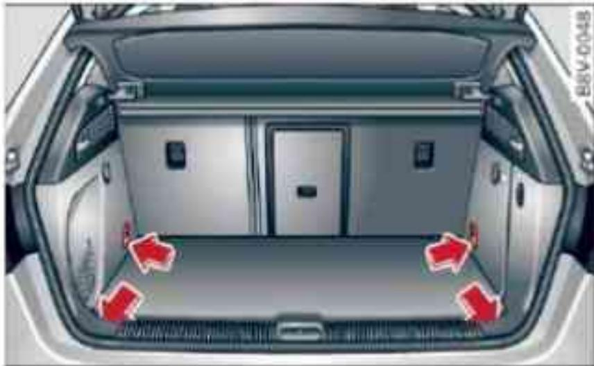
Fig. 87 Luggage compartment: Location of fastening rings (example)
