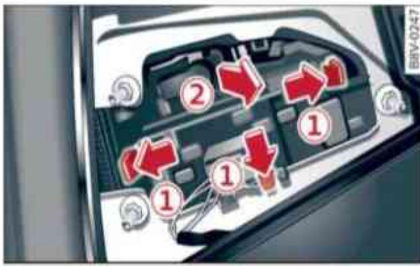
Fig. 314 Boot lid (A3 Saloon): Removing bulb carrier
