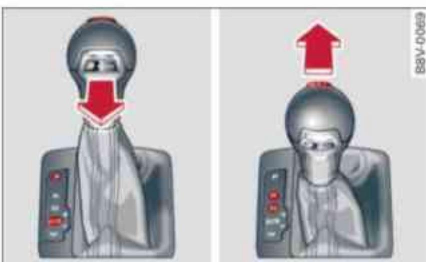
Fig. 118 Selector lever lock
