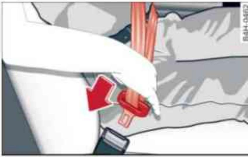
Fig. 182 Driver's seat: Belt buckle and latch plate
