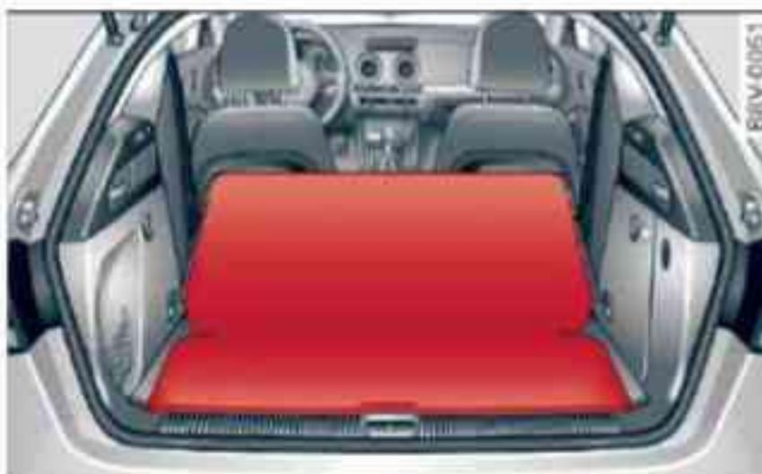
Fig. 91 Luggage compartment: Reversible floor covering with backrest folded down (example)
