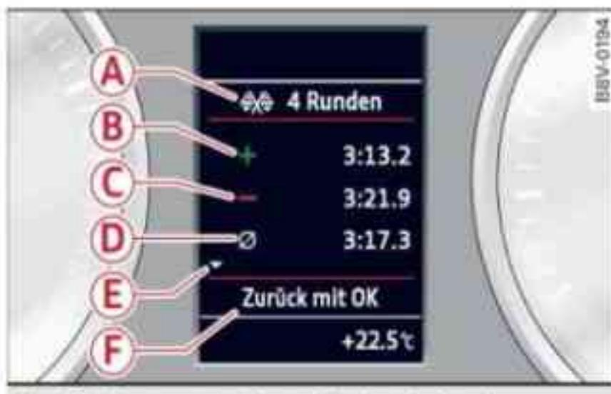
Fig. 32 Instrument cluster: Evaluating lap times
