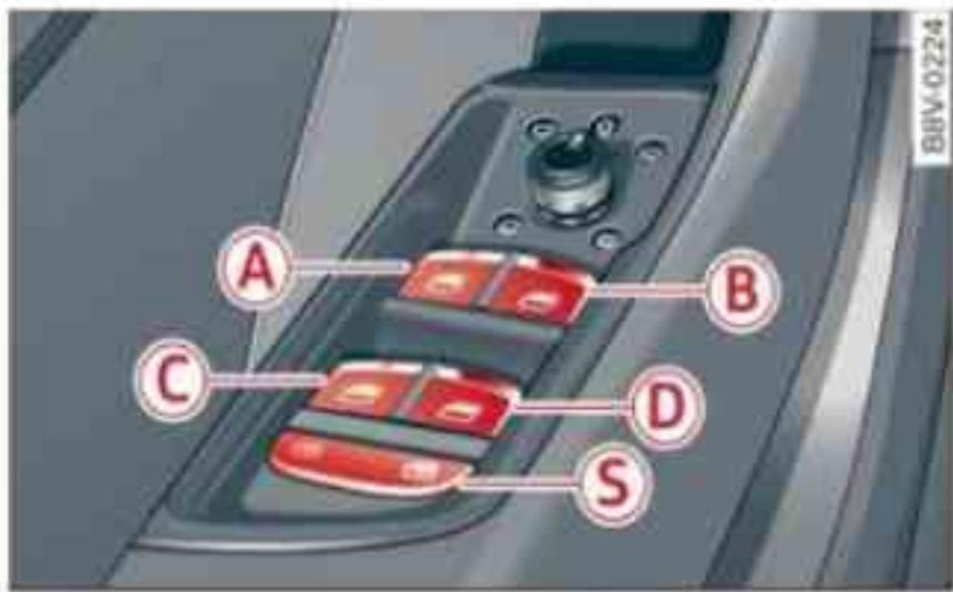
Fig. 48 Detail of the driver's door: Controls (example for A3 Sportback/A3 Saloon)
