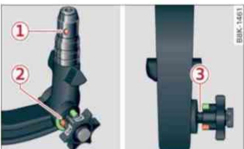
Fig. 205 Removable towing bracket: Ball joint
