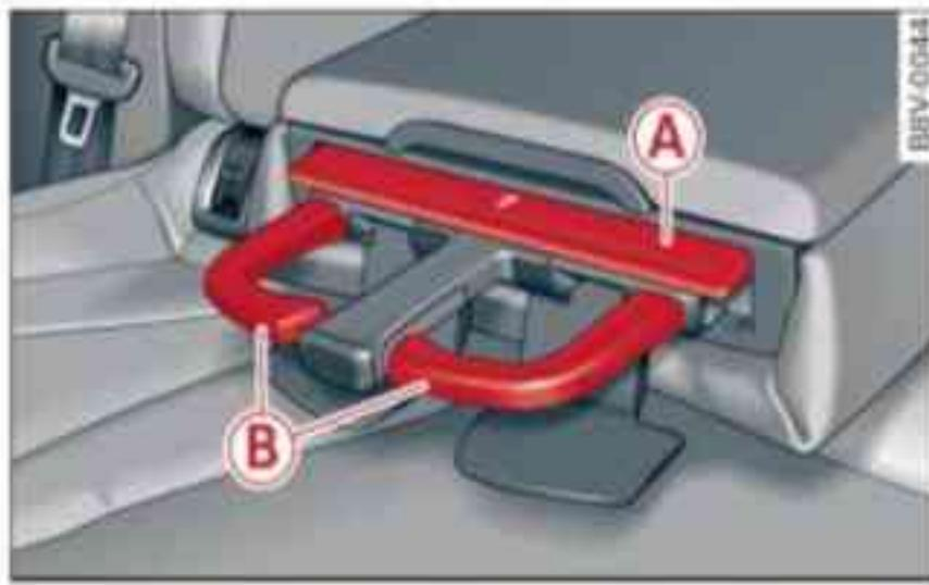
Fig. 79 Detail of the rear seat bench: Rear cup holder\*
