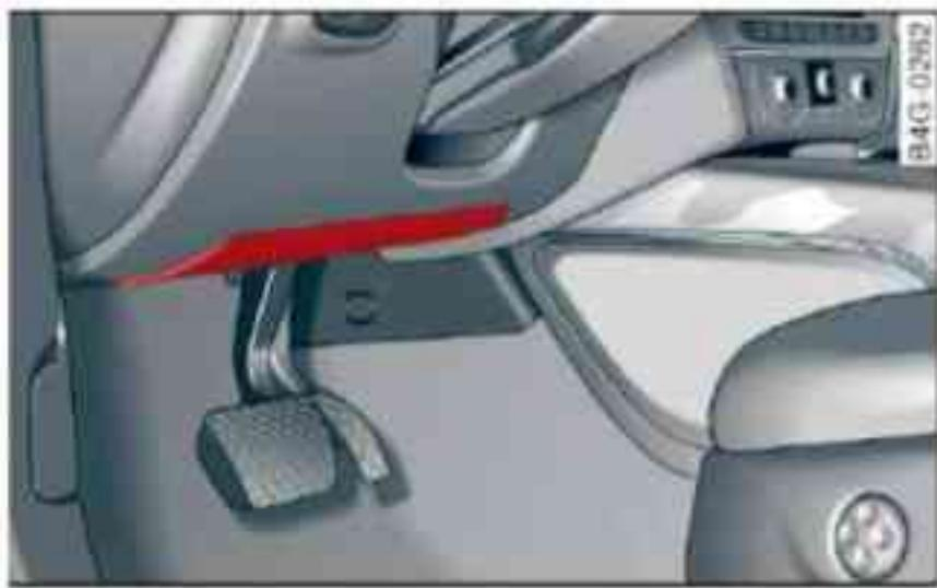
Fig. 192 Airbag (driver's side)
