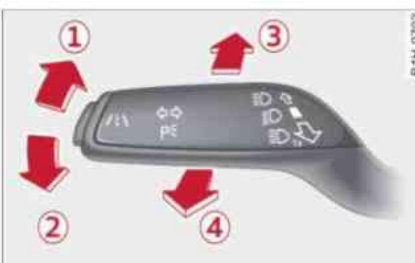
Fig. 51 Turn signal and main beam headlight lever
