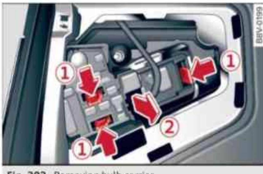
Fig. 302 Removing bulb carrier
