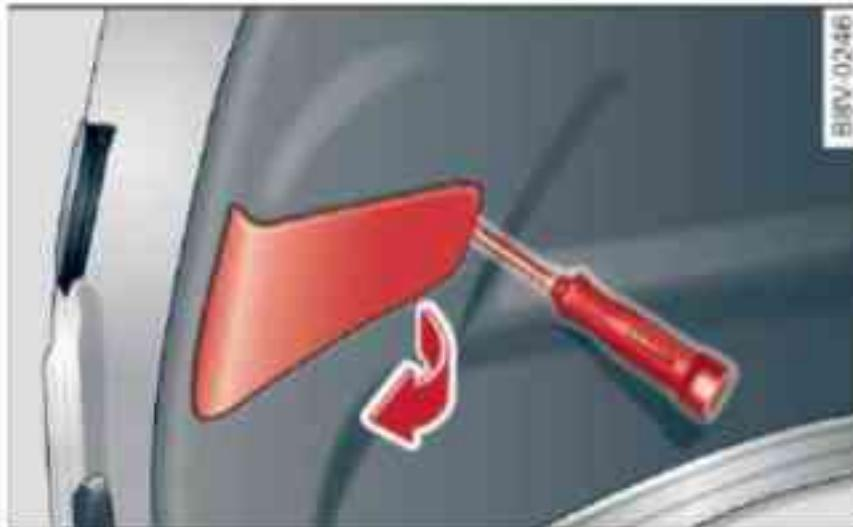
Fig. 316 Open boot lid: Removing cover from boot lid interior trim
