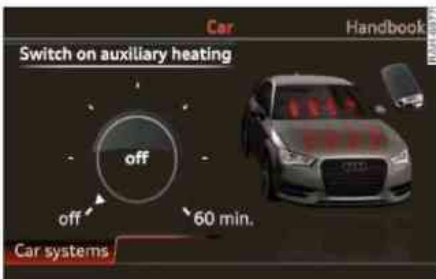
Fig. 98 MMI: Switching auxiliary heating on/off immediately
