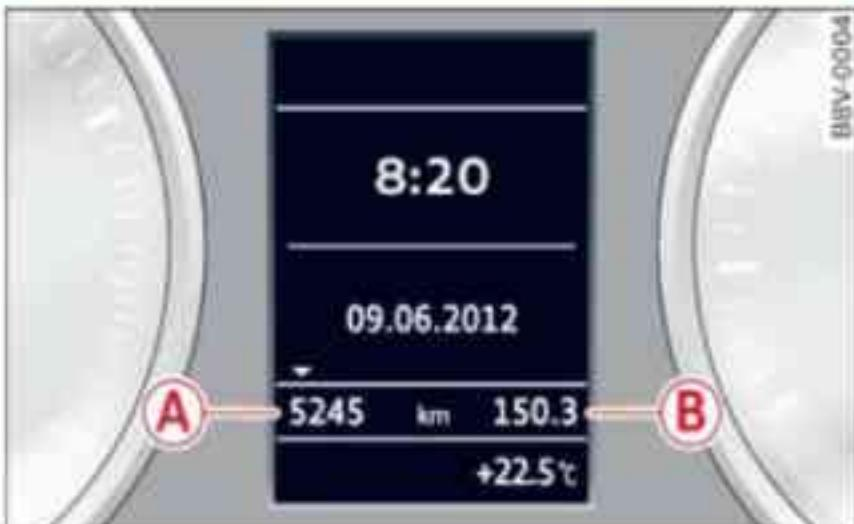
Fig. 5 Instrument cluster: Mileage recorder and reset button
