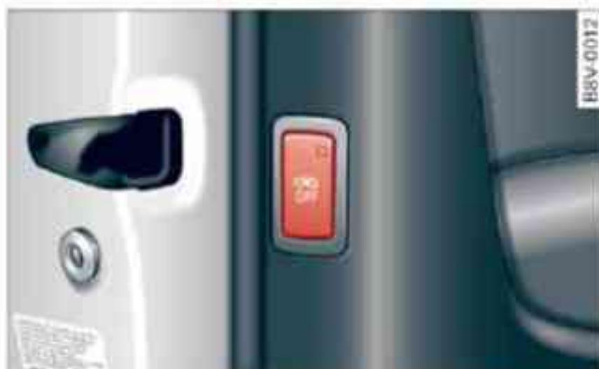
Fig. 40 Side trim in open driver's door: Button for interior monitor/tow-away protection
