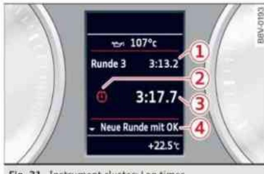
Fig. 31 Instrument cluster: Lap timer
