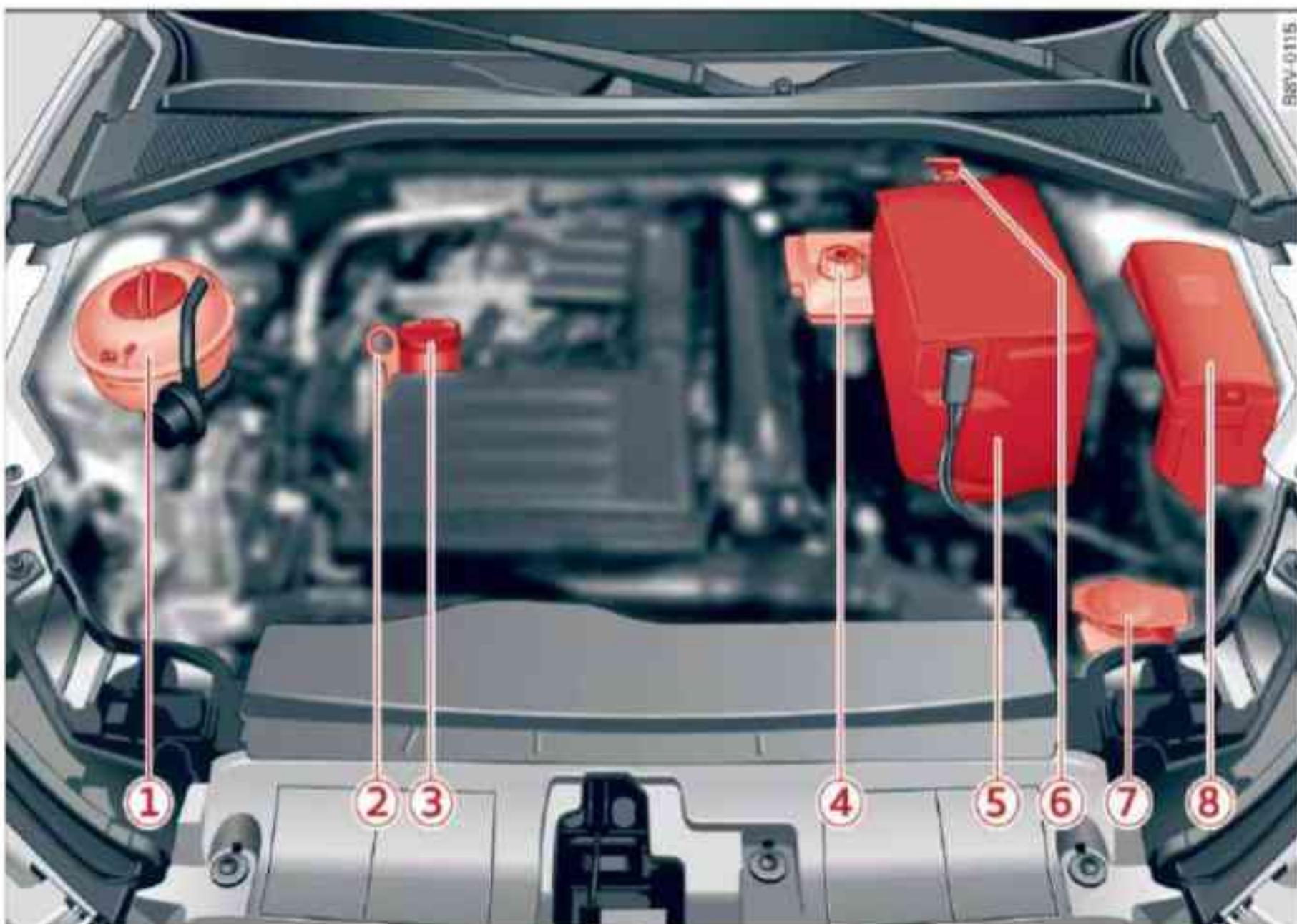
Fig. 220 Typical locations of fluid containers, engine oil dipstick and engine oil filler cap
