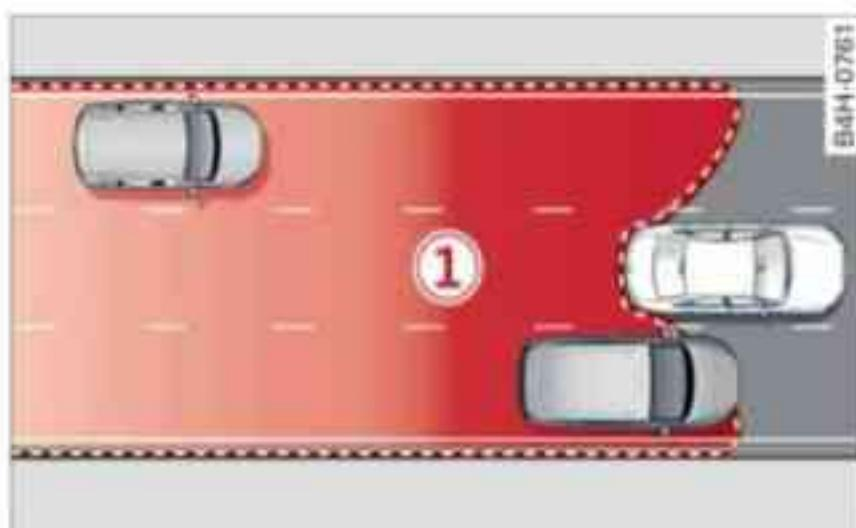
Fig. 141 Area covered by the radar sensors
