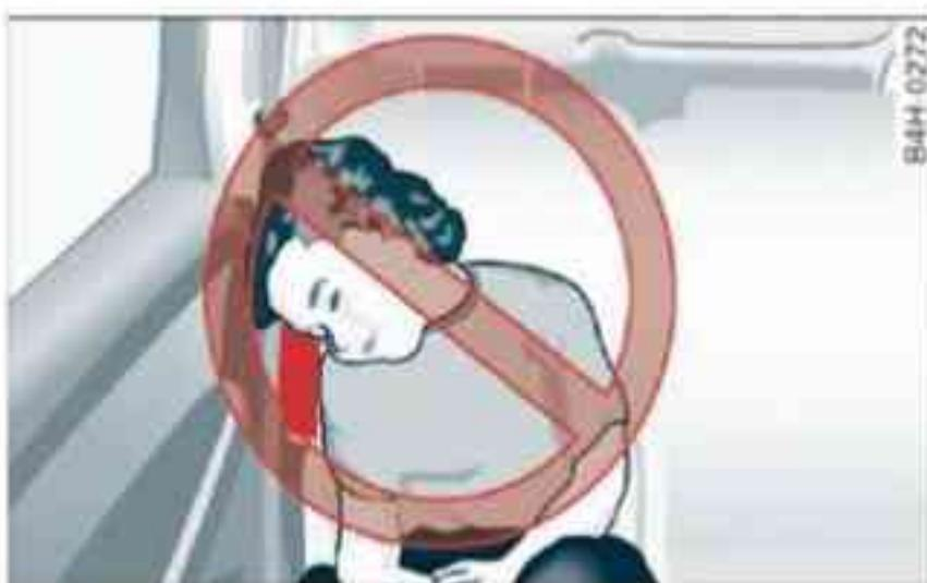
Fig. 168 Illustration of a dangerous sitting position near the opening for the side airbag
