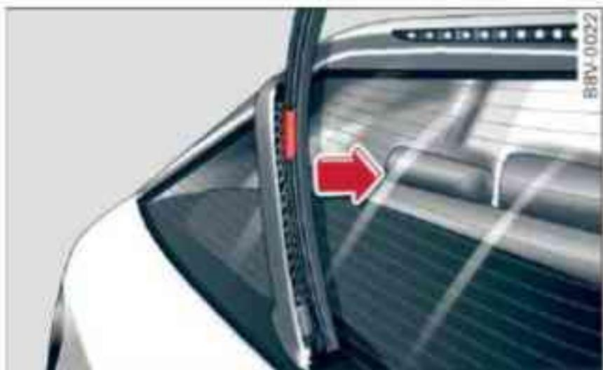
Fig. 65 Rear window wiper: Removing the wiper blade
