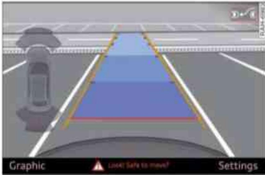
Fig. 155 MMI: Aligning the vehicle
