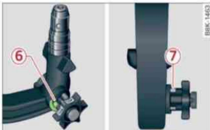
Fig. 208 Removable towing bracket: Safety check
