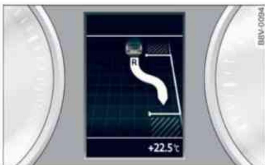
Fig. 164 Instrument cluster: Prompt to select reverse gear
