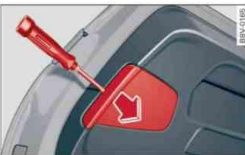
Fig. 299 Open boot lid: Removing cover from boot lid interior trim
