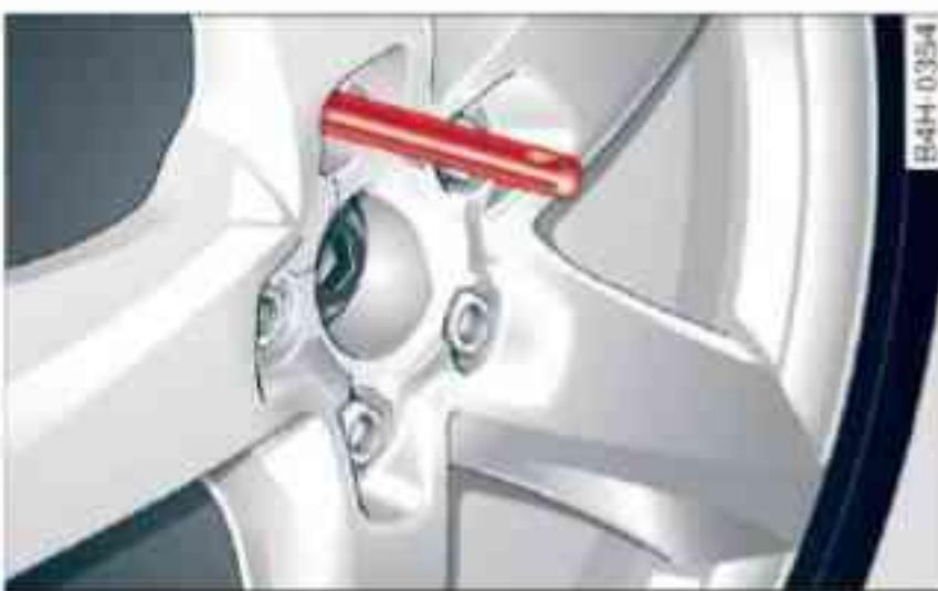
Fig. 246 Wheel: Mounting pin in wheel bolt hole nearest to the top
