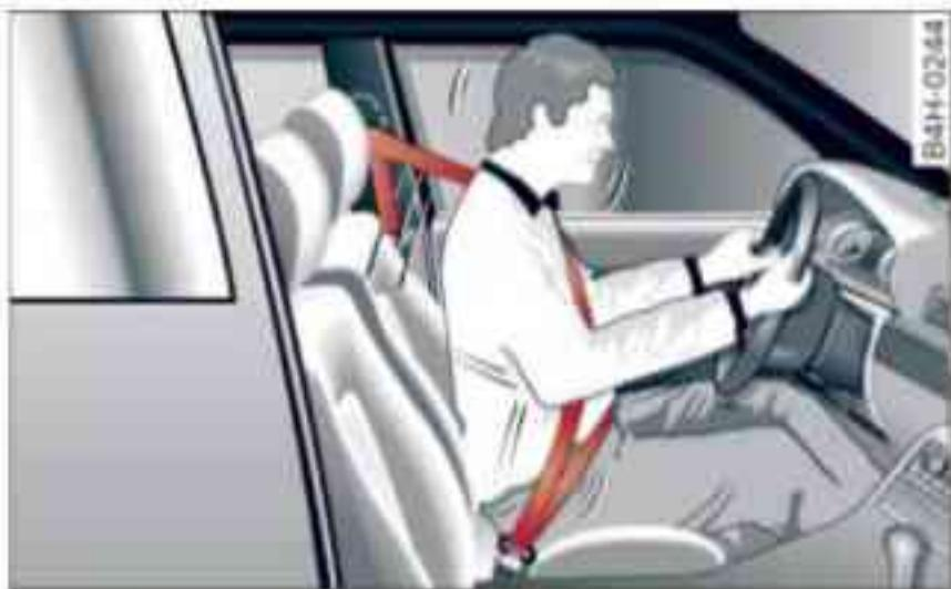
Fig. 176 Driver with properly positioned seat belt – good protection if the brakes are applied suddenly
