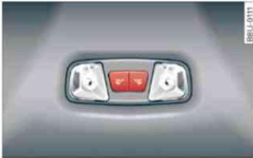
Fig. 57 Rear headliner: LED reading lights\* (example)
