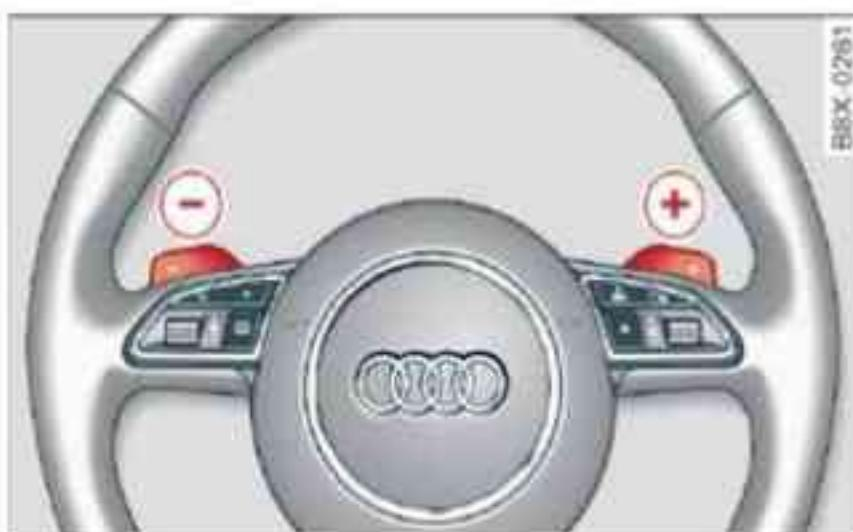
Fig. 121 Steering wheel: Manual gear selection with paddle levers\*
