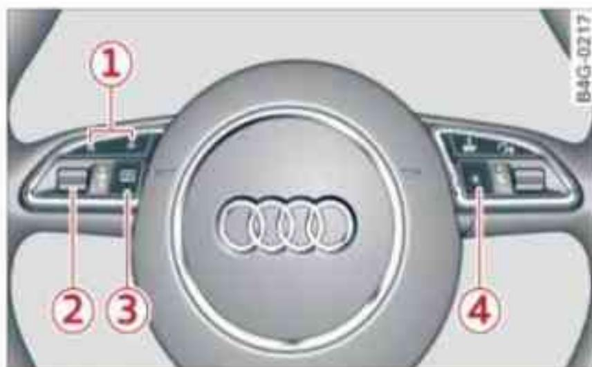
Fig. 15 Multi-function steering wheel: Driver information system controls
