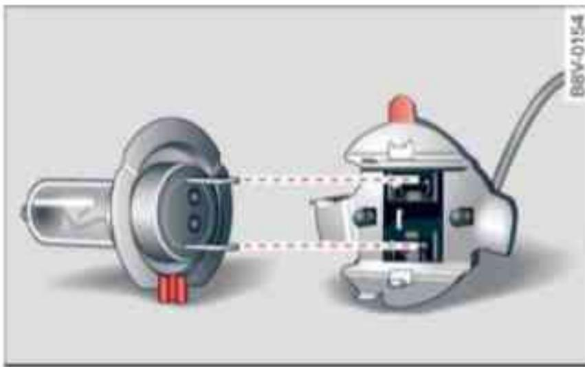
Fig. 270 Inserting the bulb correctly
