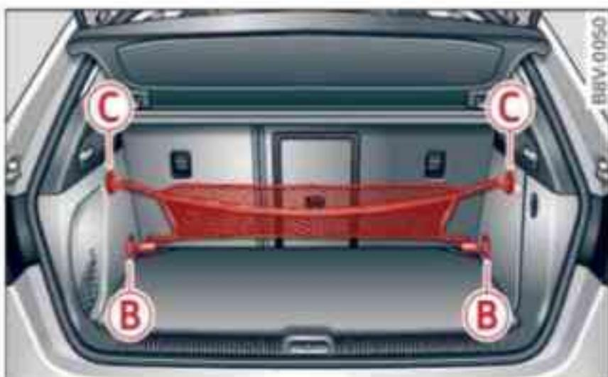
Fig. 89 Luggage compartment: Storage net hooked in place (A3/A3 Sportback)
