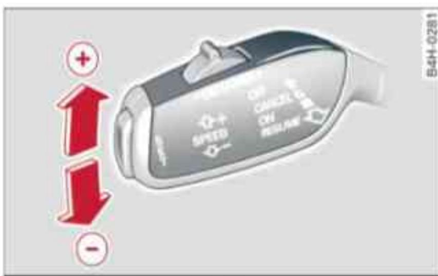
Fig. 132 Control lever: Setting a new speed
