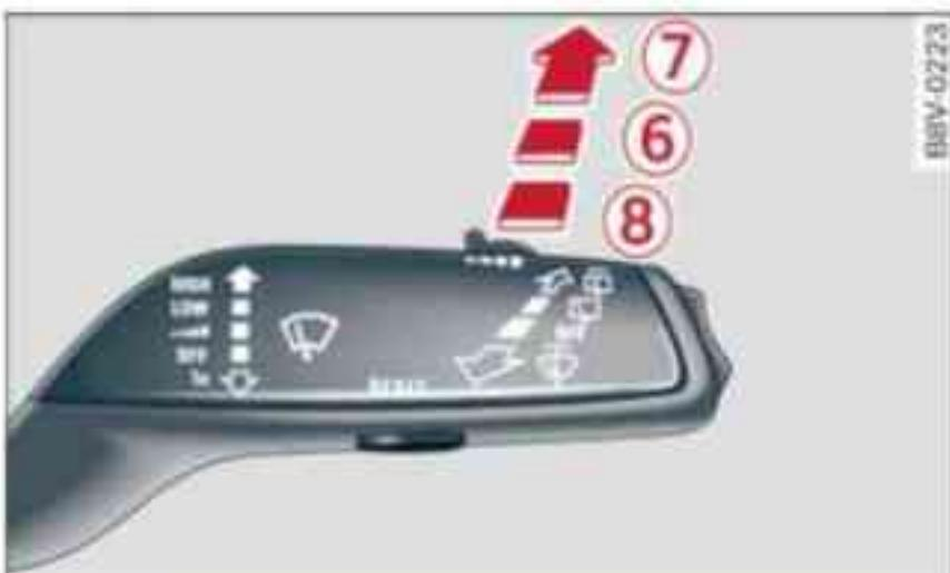
Fig. 63 Windscreen wiper lever with rear window wiper: Operating the rear wiper
