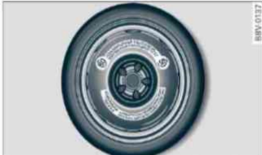
Fig. 248 Compact temporary spare wheel (example)
