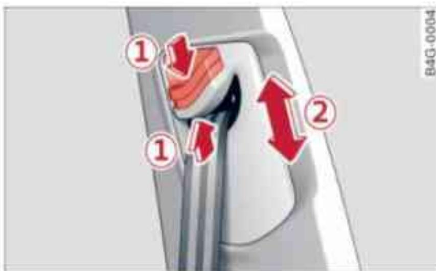
Fig. 185 Belt height adjustment for the front seats: guide fitting
