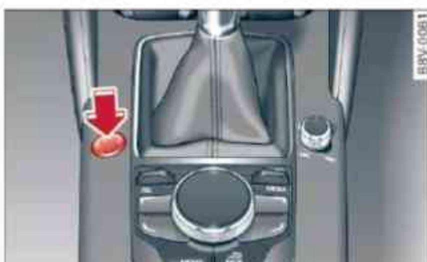
Fig. 104 Centre console: START ENGINE STOP button (vehicles with convenience key)
