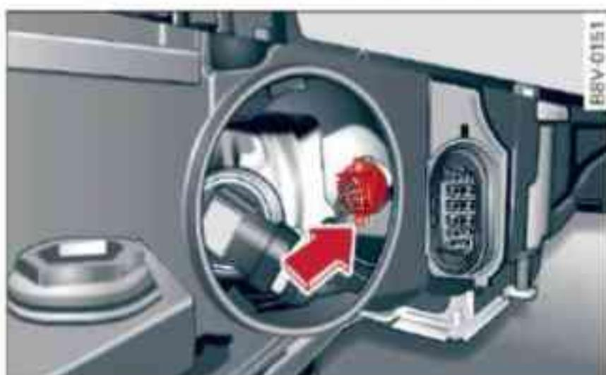
Fig. 283 Bulb housing: Tightening the bulb holder
