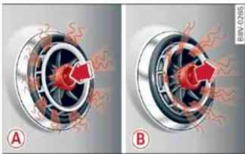
Fig. 97 Air outlet: Adjusting air flow character. A) Diffuse, B) Spot
