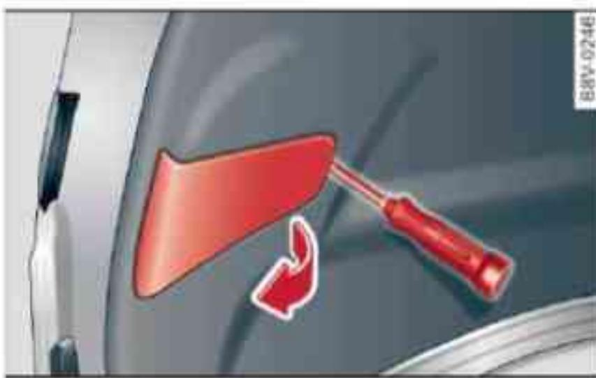
Fig. 313 Open boot lid (A3 Saloon): Removing cover from boot lid interior trim
