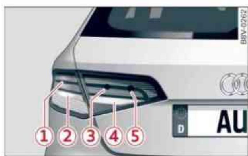
Fig. 264 Halogen system, rear light: Bulbs in side panel and boot lid
