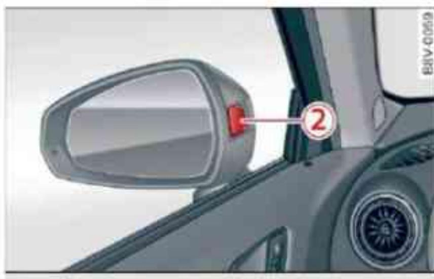
Fig. 142 Warning lamp on exterior mirror
