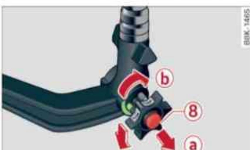
Fig. 210 Removable towing bracket: Removing the ball joint
