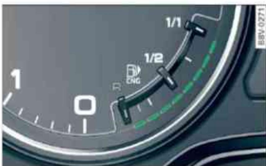
Fig. 113 Instrument cluster: Gas fuel gauge
