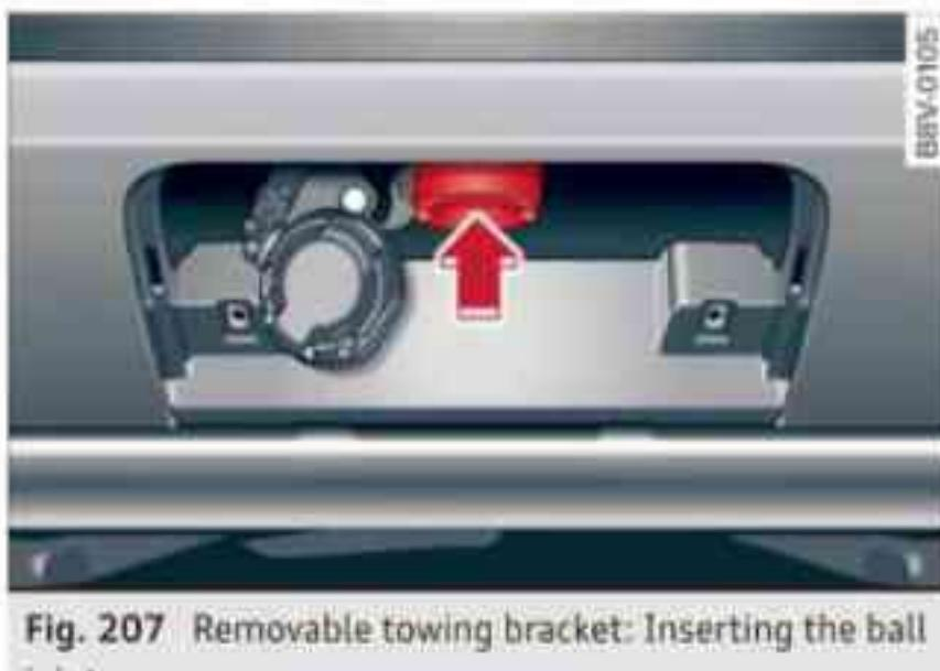
Fig. 207 Removable towing bracket: Inserting the ball joint
