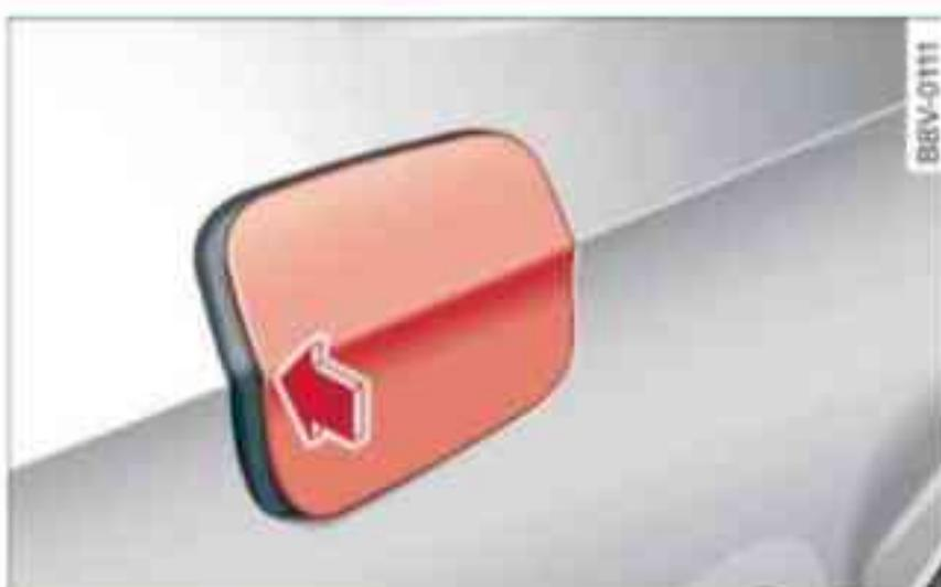
Fig. 215 Vehicle as seen from the rear right: Opening the fuel tank flap
