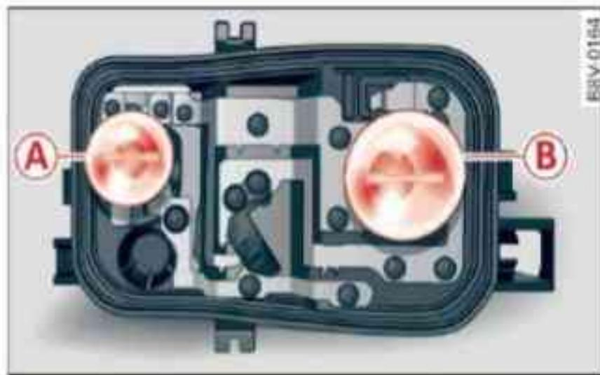
Fig. 297 Position of the bulbs on the bulb carrier (example: left rear light)
