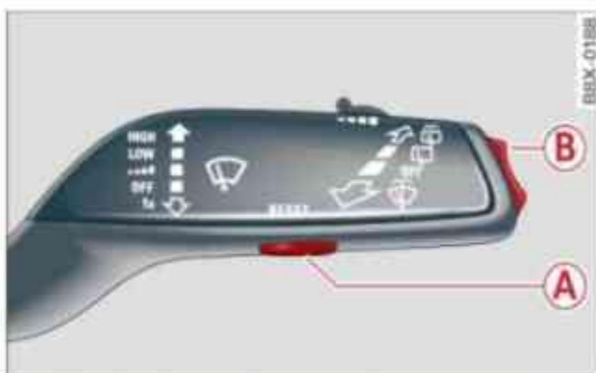
Fig. 13 Windscreen wiper lever: Driver information system controls
