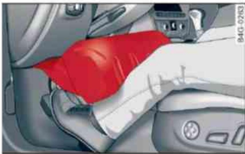
Fig. 193 Inflated airbags provide protection in a frontal collision
