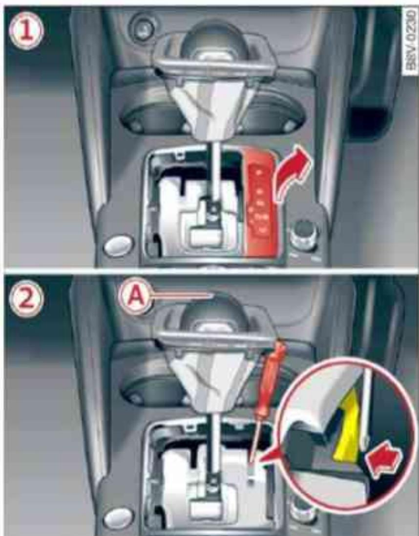
Fig. 125 Manually releasing the selector lever from position P
