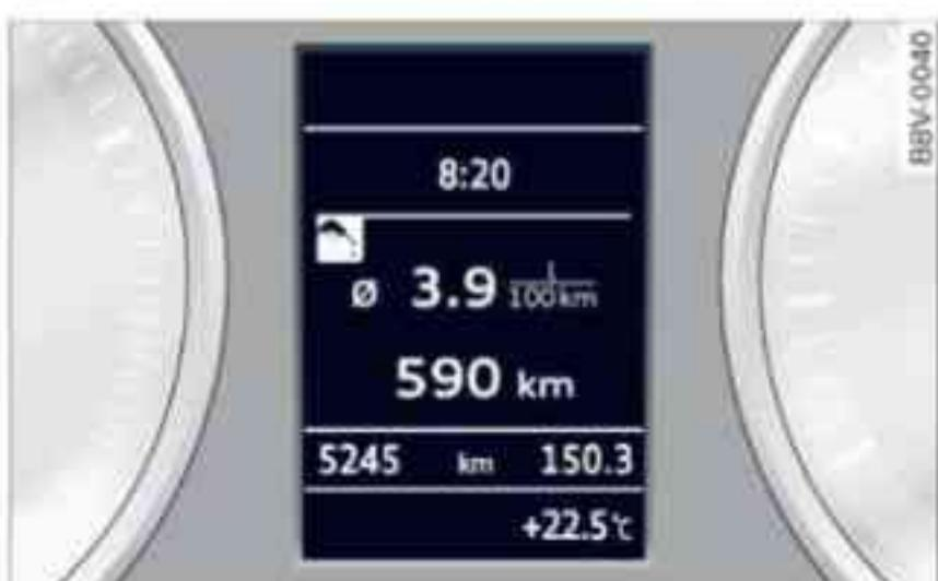
Fig. 18 Instrument cluster: Efficiency programme
