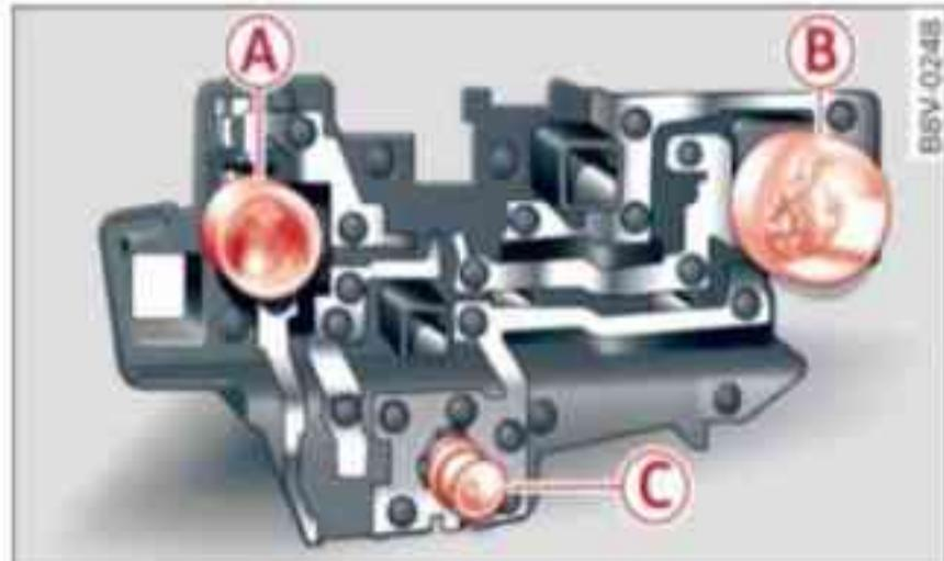
Fig. 315 Position of the bulbs on the bulb carrier (example for inner left rear light)
