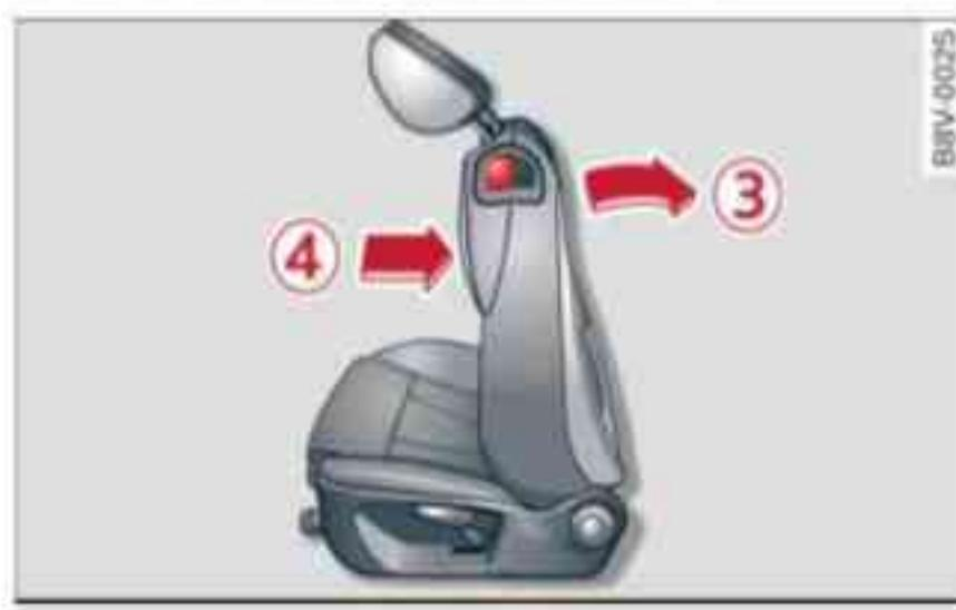
Fig. 69 Tips for using the easy entry feature, seat adjustment with memory function
