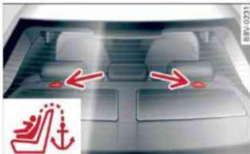
Fig. 172 Rear seat bench (A3 Saloon): Top tether anchorages
