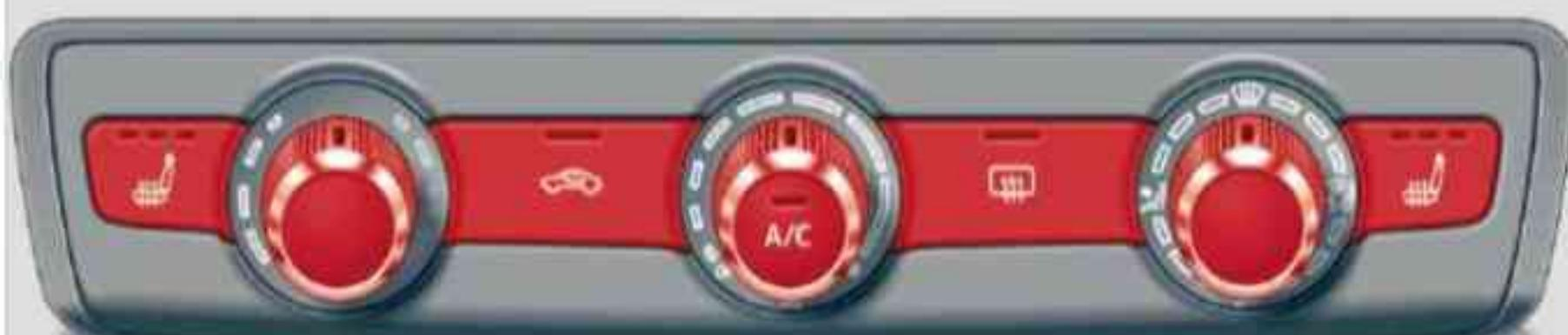
Fig. 94 Heating/ventilation system or manual air conditioner\*: Controls
