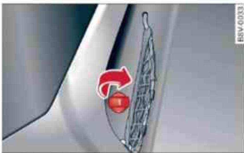
Fig. 77 Side trim in luggage compartment: 12 Volt socket\* (example)
