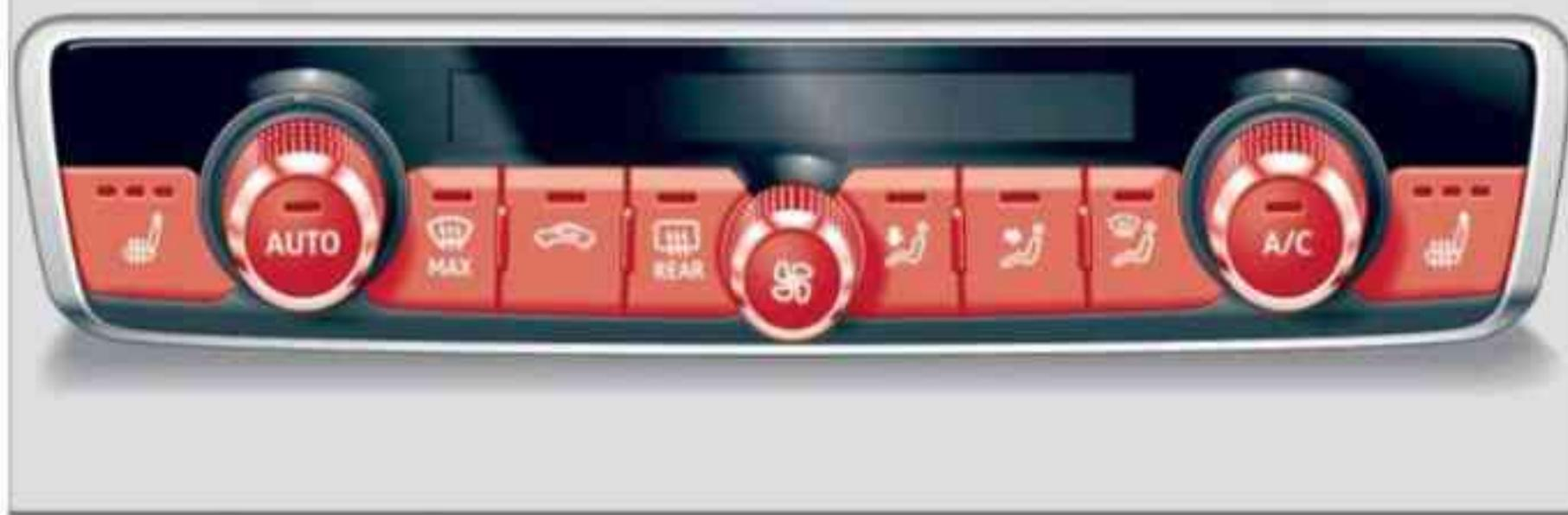
Fig. 95 Automatic air conditioner: Controls
