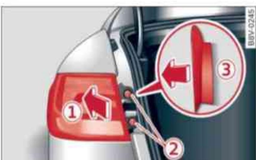
Fig. 312 Fitting the rear light
