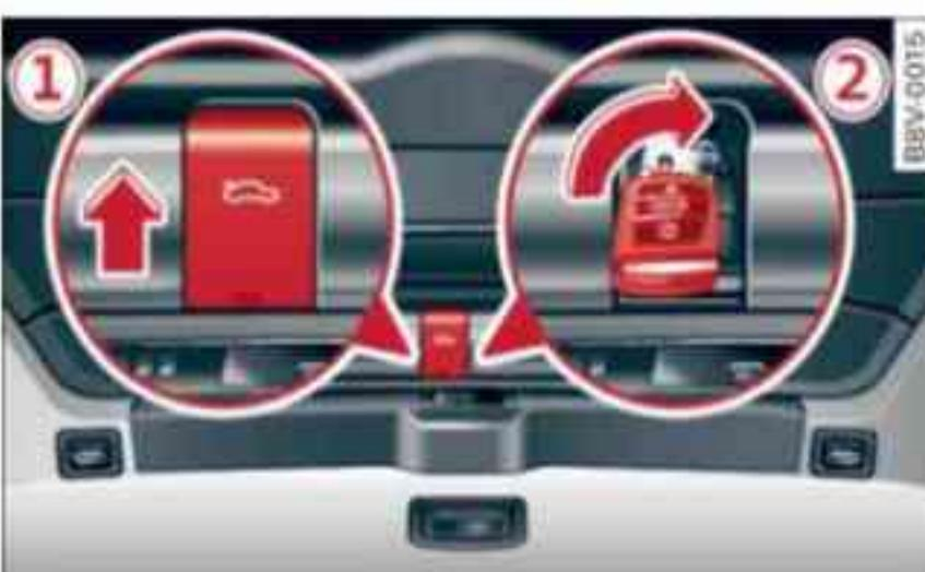
Fig. 44 (A3/A3 Sportback) Detail of inside of boot lid: Access to manual release
