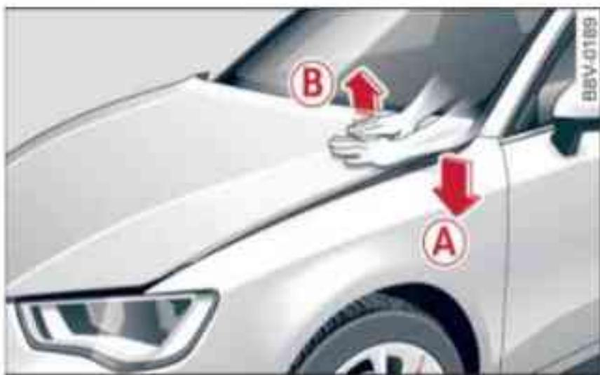
Fig. 175 Pressing back/checking the bonnet
