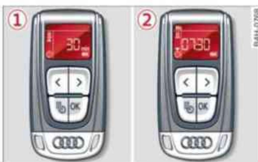
**Fig. 100** Remote control for auxiliary heating: ① switching on immediately ② setting the timer
