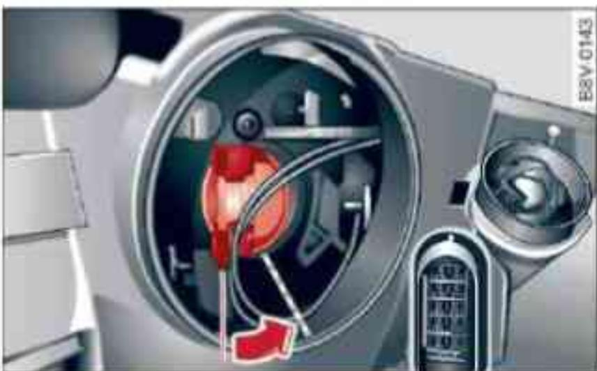
Fig. 273 Bulb holder for main beam headlights/daytime running lights
