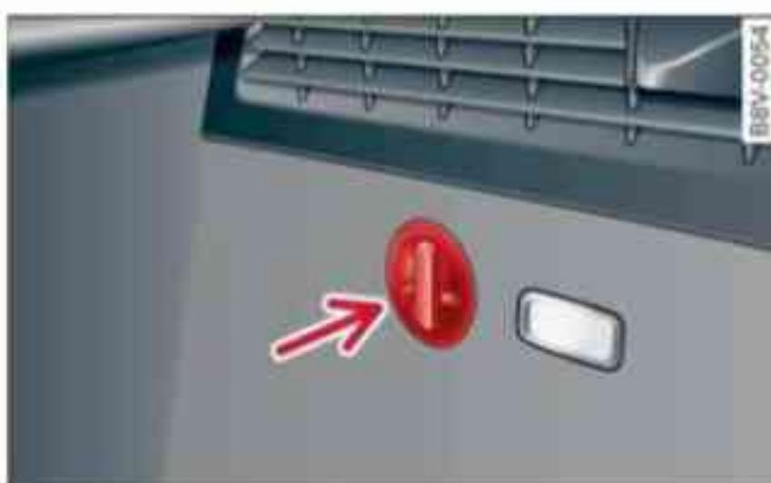
Fig. 90 Luggage compartment: Retaining hook (example of right side)
