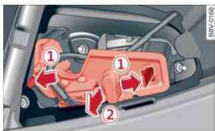
Fig. 305 Removing bulb carrier
