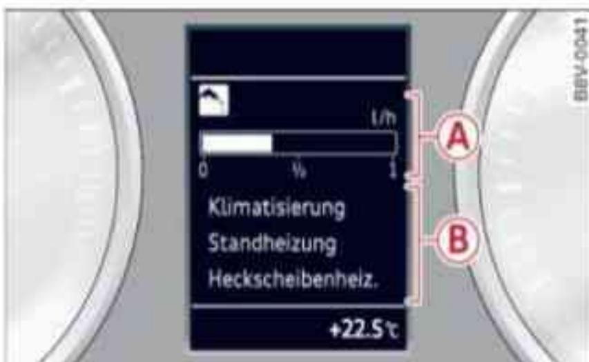
Fig. 21 Instrument cluster: Auxiliaries
