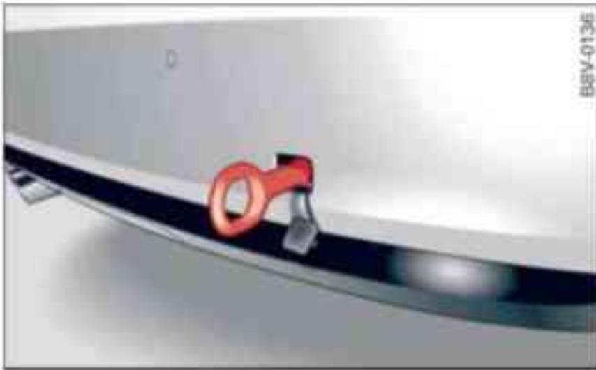
Fig. 254 Right side of the rear bumper: Towline anchorage screwed in
