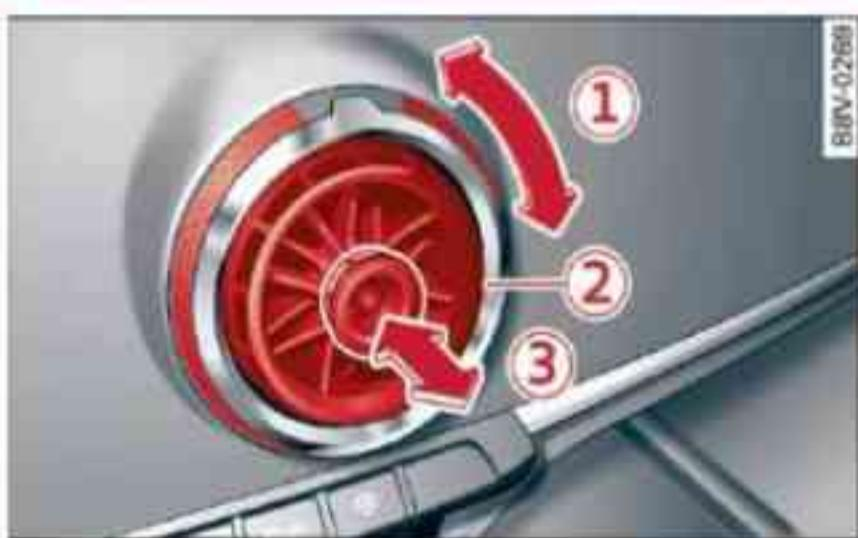
Fig. 96 Dashboard: Adjusting air outlet
