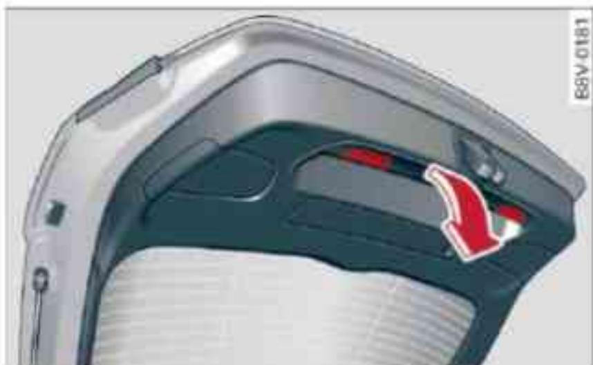
Fig. 43 Boot lid/handle on inside (example): Closing
