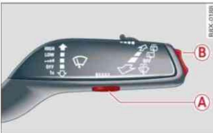
Fig. 27 Windscreen wiper lever: Controls
