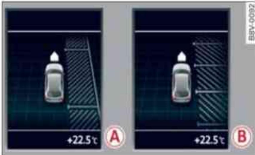
Fig. 162 Instrument cluster: Looking for a parking space. (A) parallel to the roadside, (B) perpendicular to the roadside
