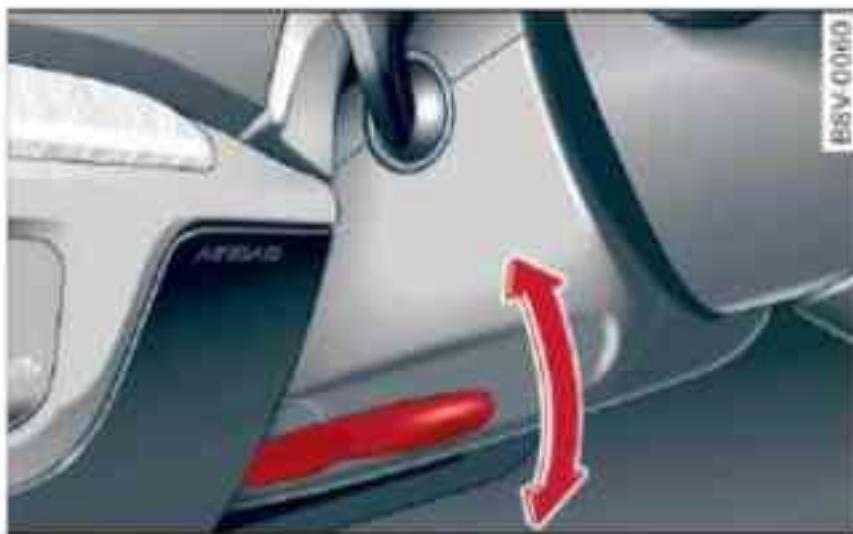
Fig. 102 Steering column: Lever for steering column adjustment
