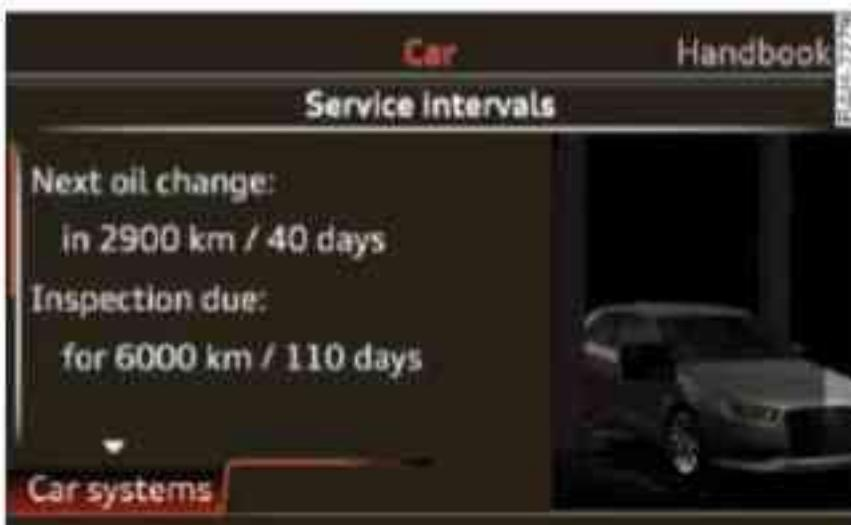
Fig. 10 MMI\* system display on dashboard: Service interval display (example)
