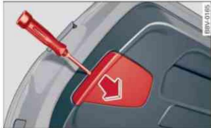
Fig. 304 Open boot lid: Removing cover from boot lid interior trim
