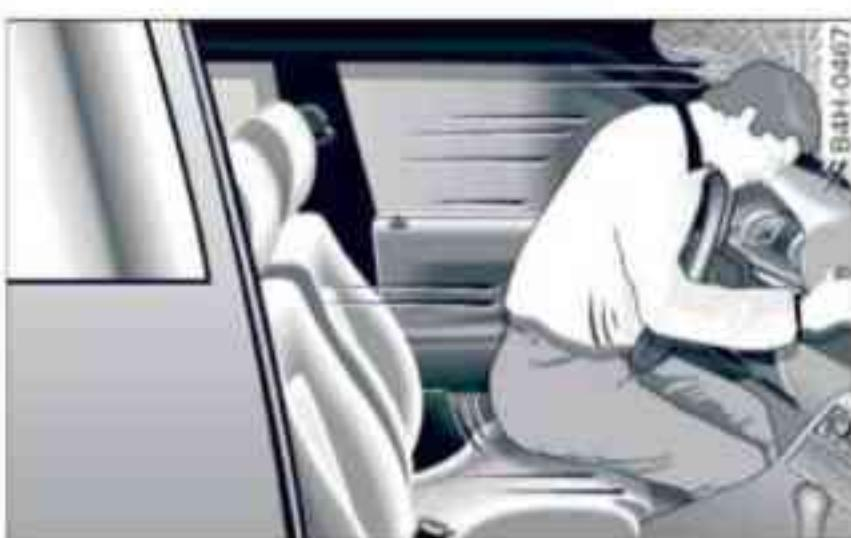
Fig. 179 A driver not wearing a seat belt can be thrown forwards
