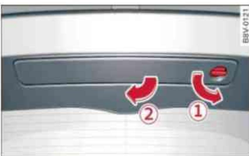
Fig. 232 A3/A3 Sportback with boot lid open: warning triangle
