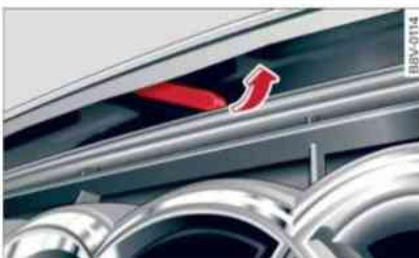
Fig. 219 Release catch under the bonnet
