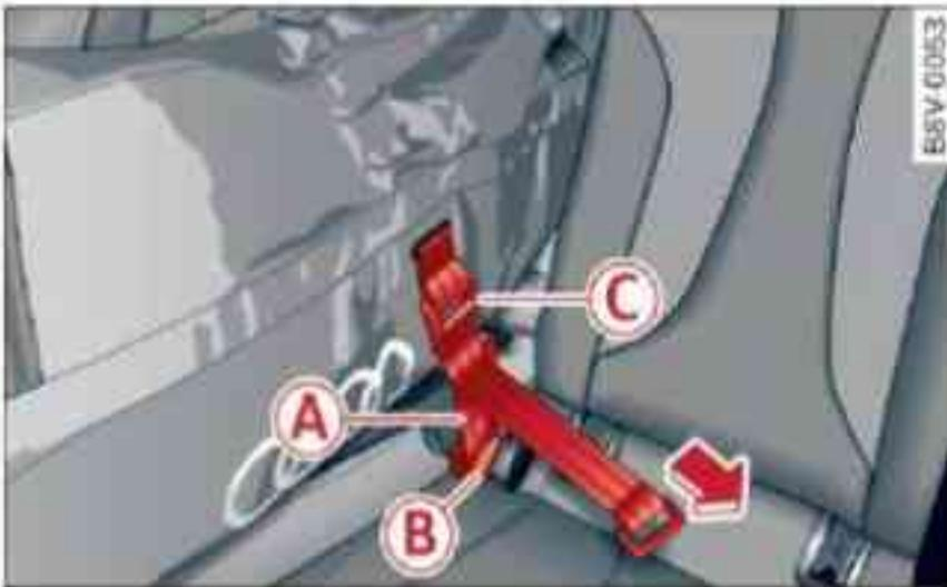
Fig. 93 Rear seat: Securing the bag
