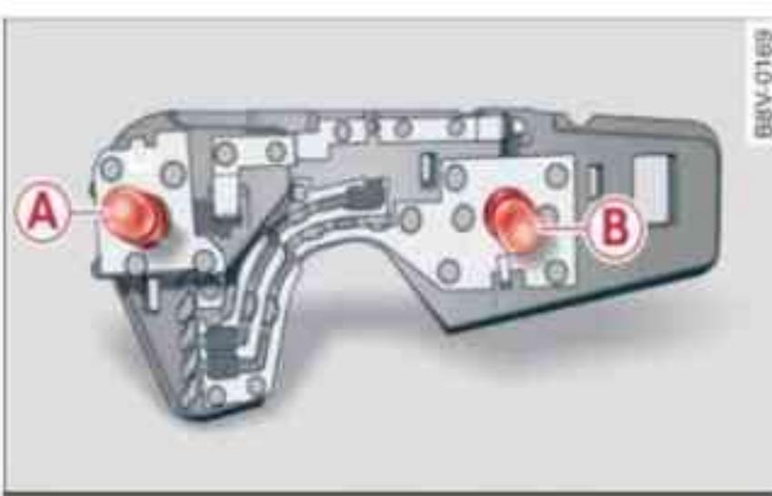
Fig. 306 Position of the bulbs on the bulb carrier (example: inner left rear light)
