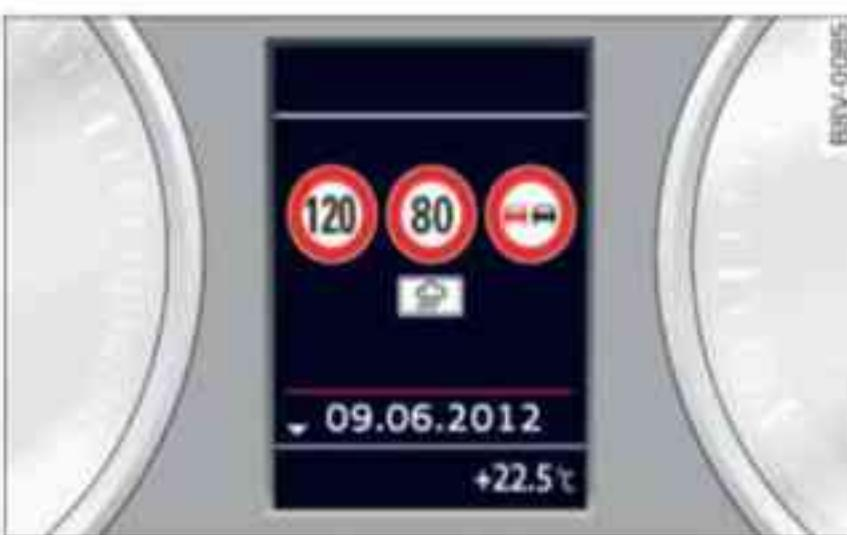
Fig. 24 Instrument cluster: Traffic sign recognition (example)
