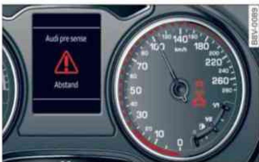
Fig. 136 Instrument cluster: Collision warning
