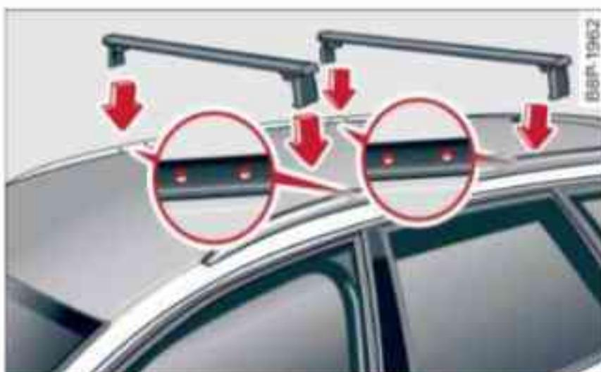
Fig. 83 A3 Sportback with roof railings: Attachment points for roof carrier
