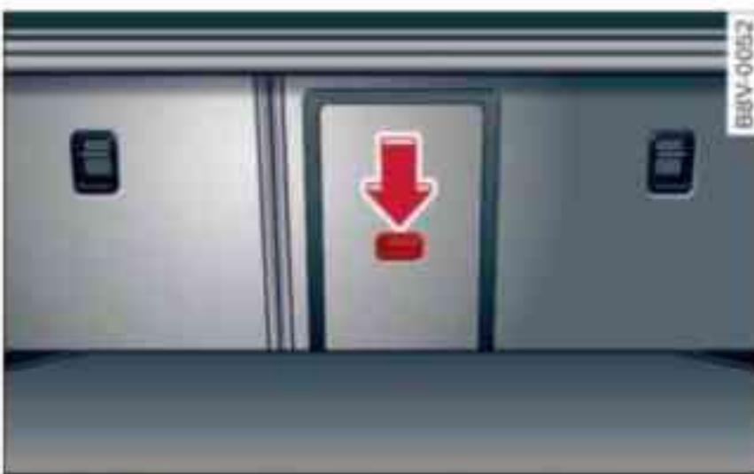
Fig. 92 Backrest: Cover of load-through hatch
