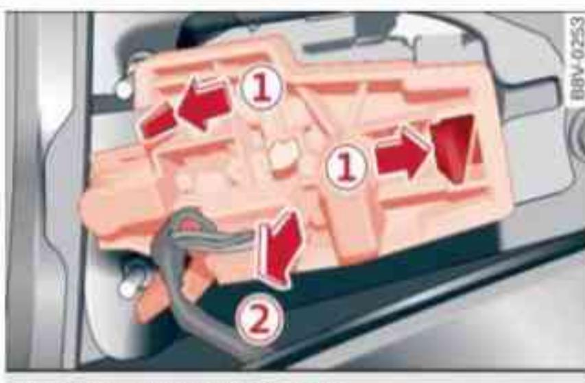
Fig. 317 Removing bulb carrier
