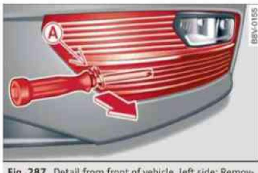
Fig. 287 Detail from front of vehicle, left side: Removing trim
