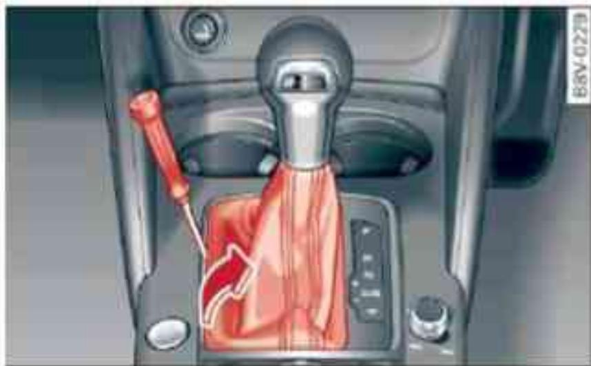
Fig. 124 Selector lever: Removing the cover
