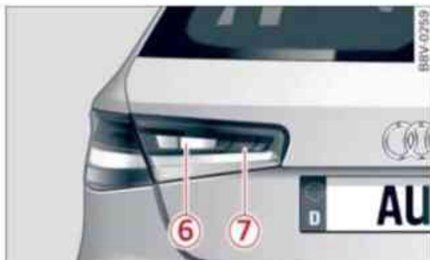
Fig. 263 Xenon/LED system, rear light: Bulbs in side panel and boot lid
