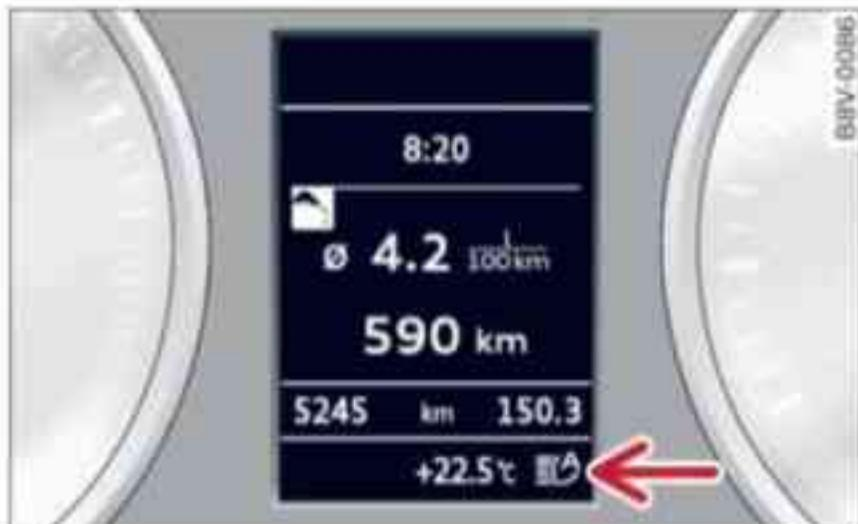
Fig. 53 Instrument cluster: Indicator lamp for main beam assist
