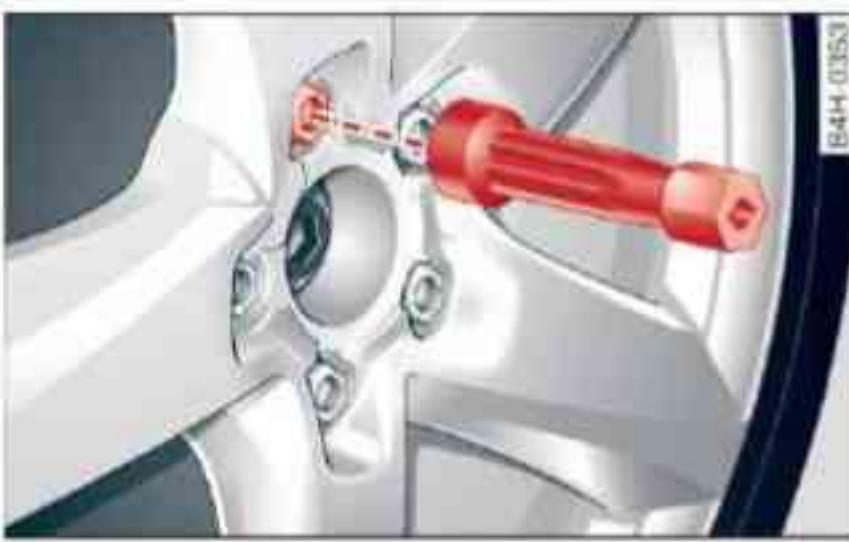
Fig. 245 Wheel: Hexagonal socket for turning wheel bolts
