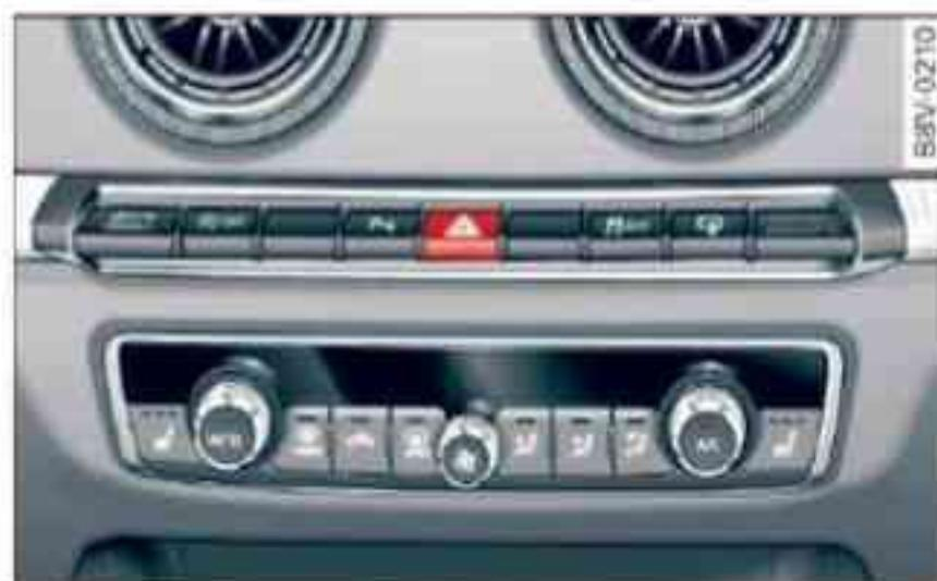
Fig. 55 Dashboard: Switch for hazard warning lights
