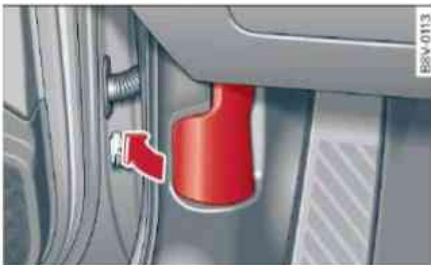
Fig. 218 Detail of footwell on driver's side: Release lever
