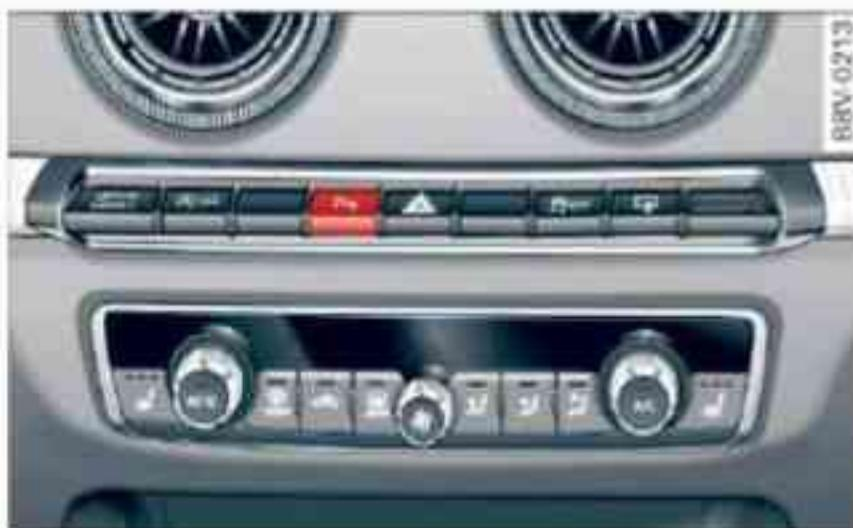
Fig. 148 Centre console: Switch for parking aid
