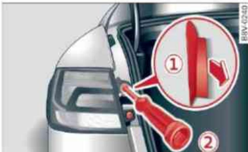
Fig. 307 Releasing rear light (example on left side)
