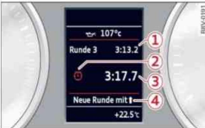
Fig. 28 Instrument cluster: Lap timer
