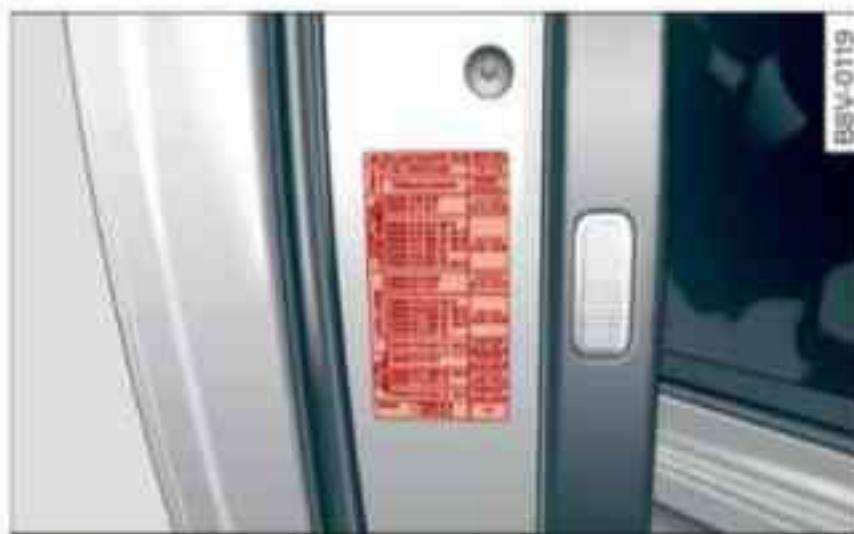
Fig. 227 Open driver's door (LHD vehicle): Sticker listing tyre pressures
