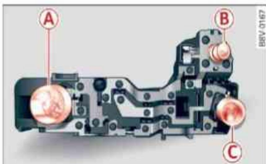
Fig. 303 Position of the bulbs on the bulb carrier (example: inner left rear light)
