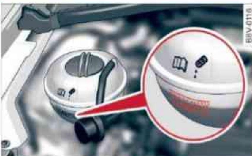
Fig. 223 Engine compartment: Markings on coolant expansion tank
