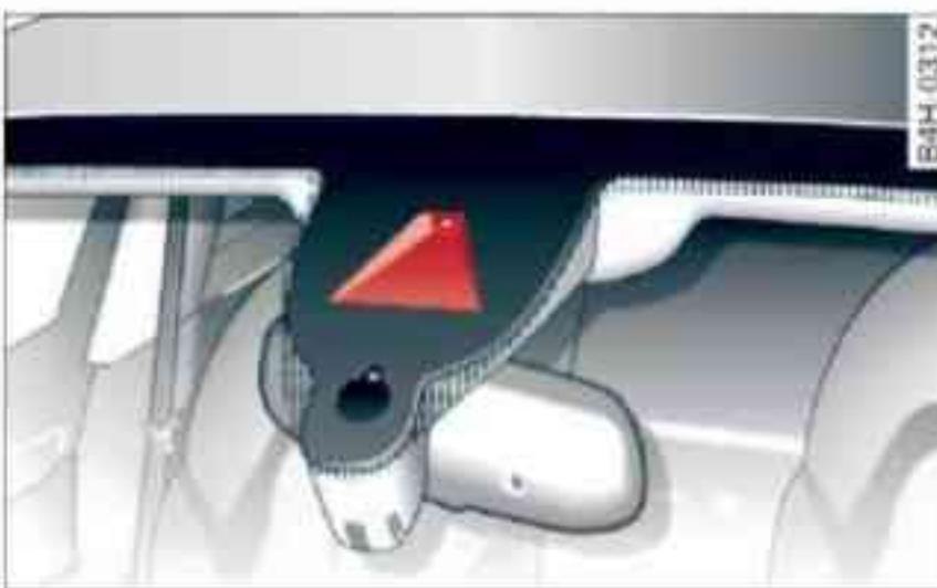
Fig. 25 Windscreen: Camera window for traffic sign recognition
