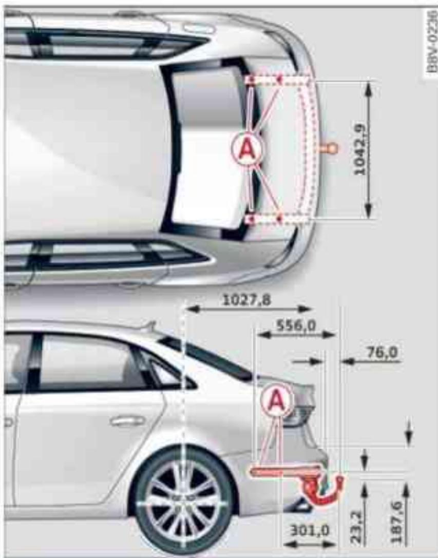
Fig. 214 A3 Saloon: Positions of securing points (viewed from above and from side)
