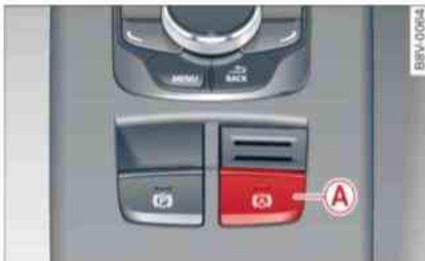
Fig. 107 Section of centre console: Button for hold assist
