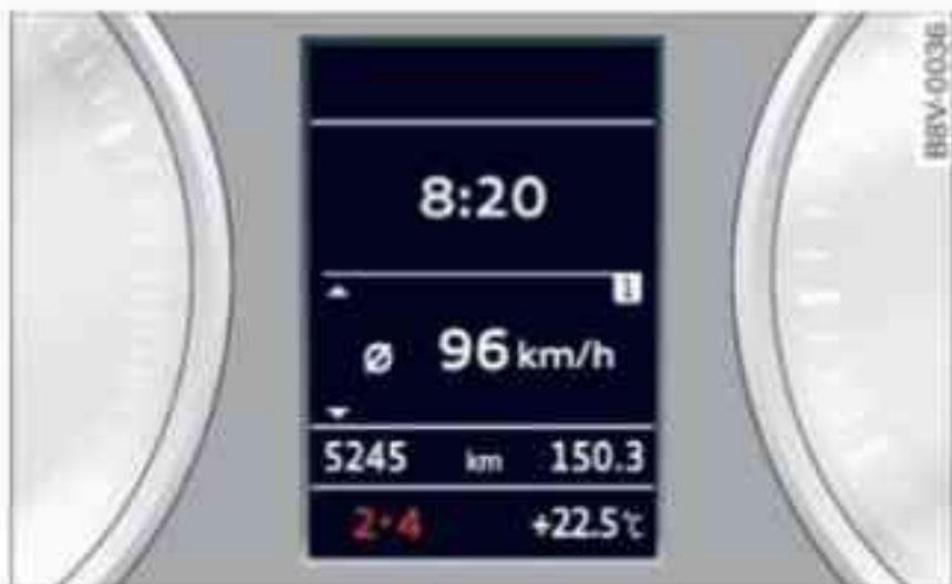
Fig. 7 Instrument cluster: Gear-change indicator (for manual gearbox)
