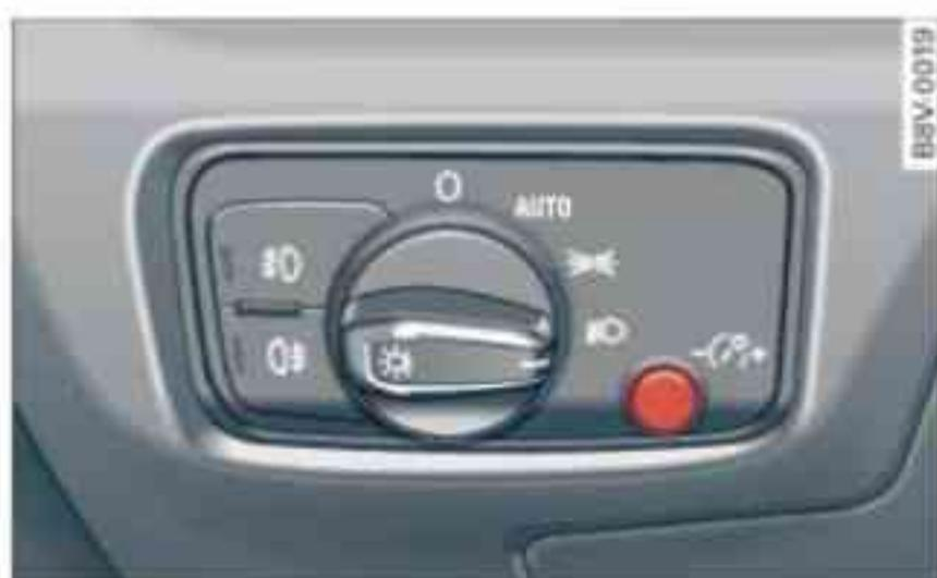
Fig. 58 Instrument lighting
