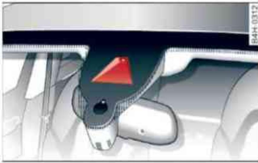
Fig. 138 Windscreen: Camera window for active lane assist
