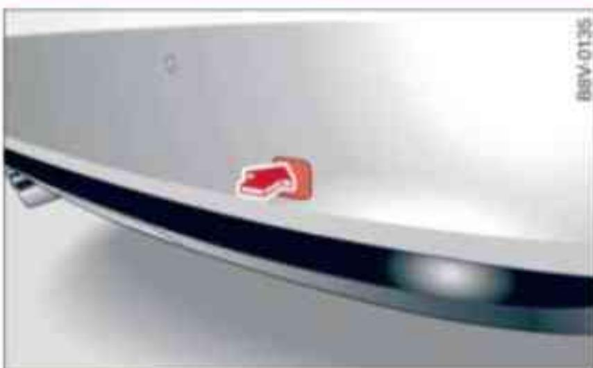
Fig. 253 Right side of the rear bumper: Cover cap
