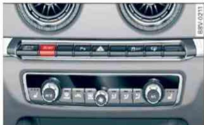
Fig. 111 Centre console: Switch for start/stop system
