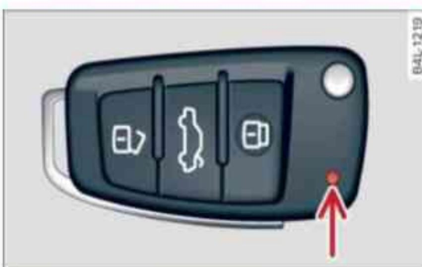
Fig. 34 Remote control key: LED
