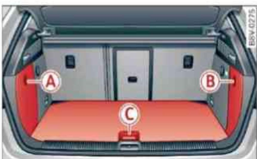
Fig. 235 Luggage compartment (example): Stowing the tools, tyre repair kit and jack\*
