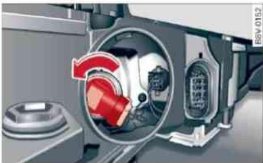
Fig. 285 Bulb holder for turning light
