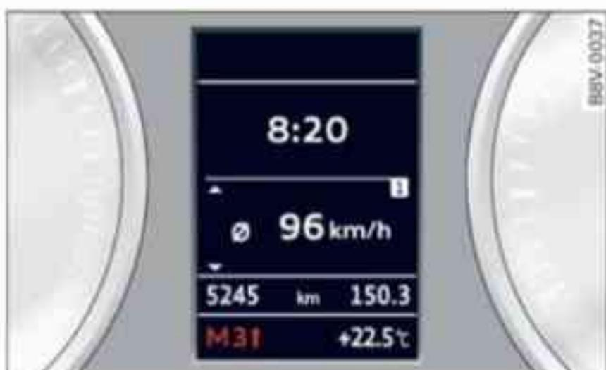
Fig. 8 Instrument cluster: Gear-change indicator in tiptronic mode (for automatic gearbox)
