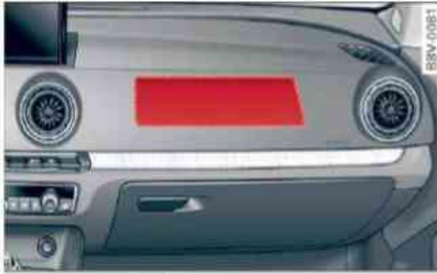
Fig. 189 Dashboard: Front passenger's airbag
