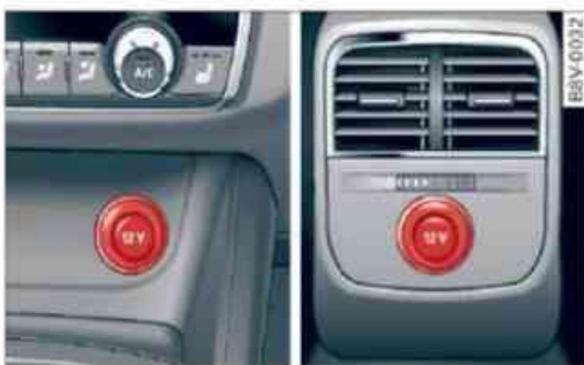
Fig. 76 Centre console: 12 Volt socket (front/rear)
