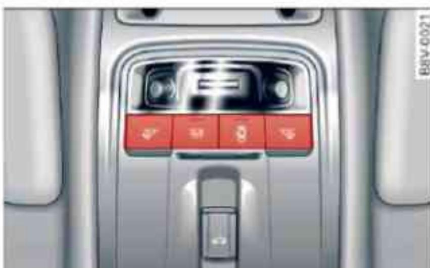
Fig. 56 Front headliner: Switches for interior lights (example)
