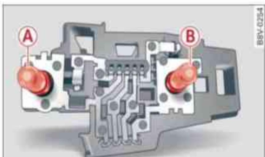
Fig. 318 Position of the bulbs on the bulb carrier (example for inner left rear light)
