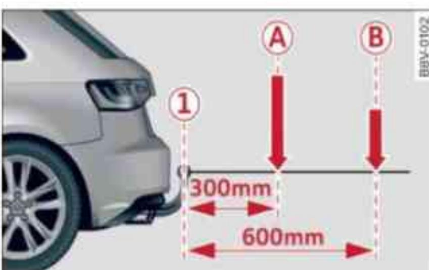
Fig. 201 Load distribution of equipment and accessories (illustration shows an example vehicle)
