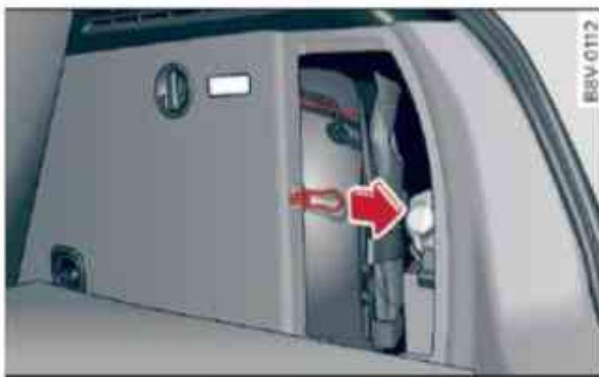
Fig. 217 Luggage compartment (rear right): Manual release (example)
