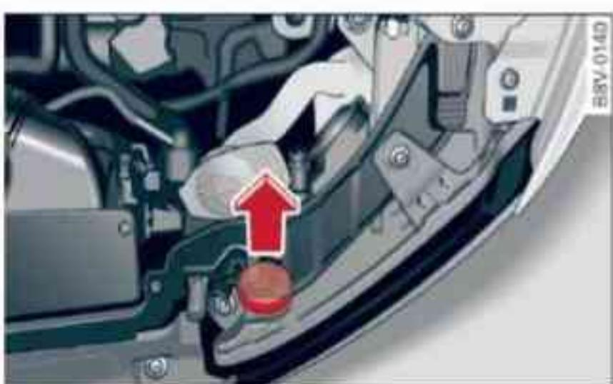
Fig. 278 Engine compartment: Removing cover
