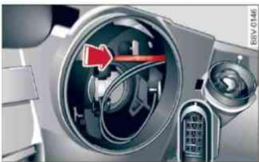
Fig. 277 Bulb housing: Inserting the bulb holder
