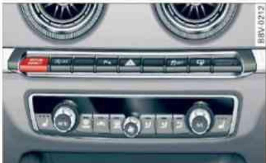
Fig. 145 Centre console: Button for drive select
