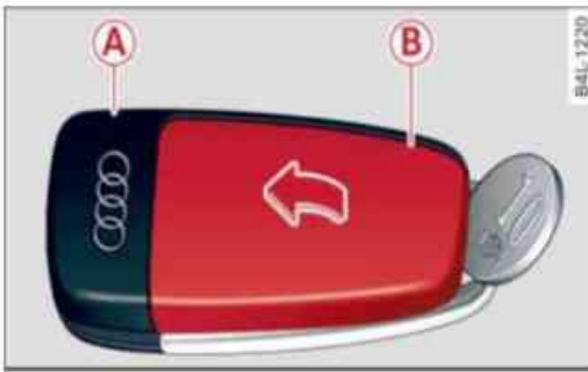
Fig. 35 Remote control key: Opening the cover
