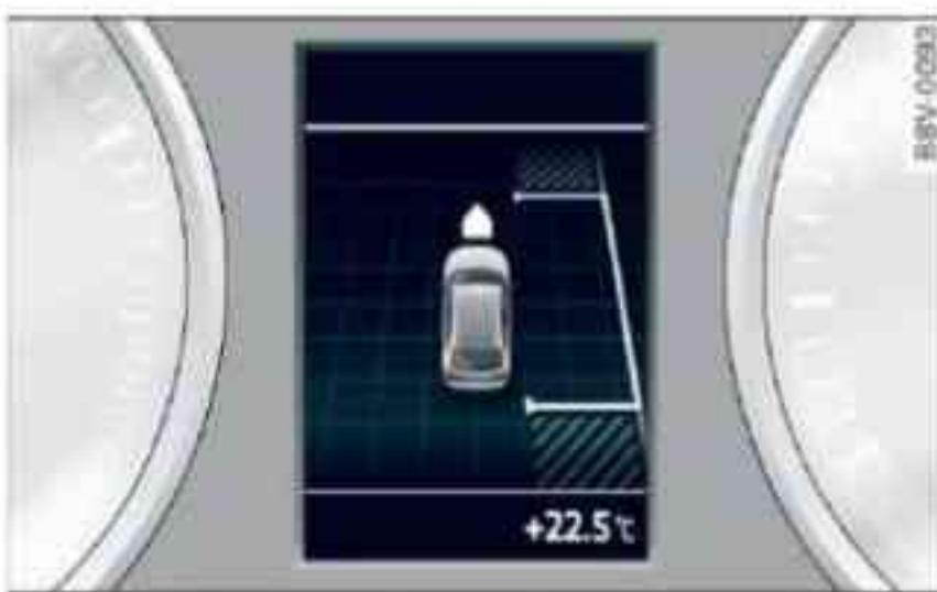
Fig. 163 Instrument cluster: Prompt to keep driving forwards (a parking space has been detected)
