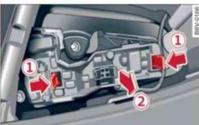
Fig. 300 Removing bulb carrier
