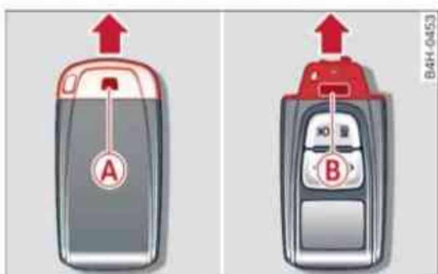
Fig. 101 Remote control: Changing battery
