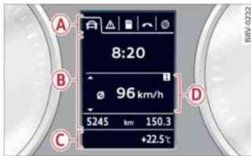
Fig. 14 Instrument cluster: Driver information system (example)
