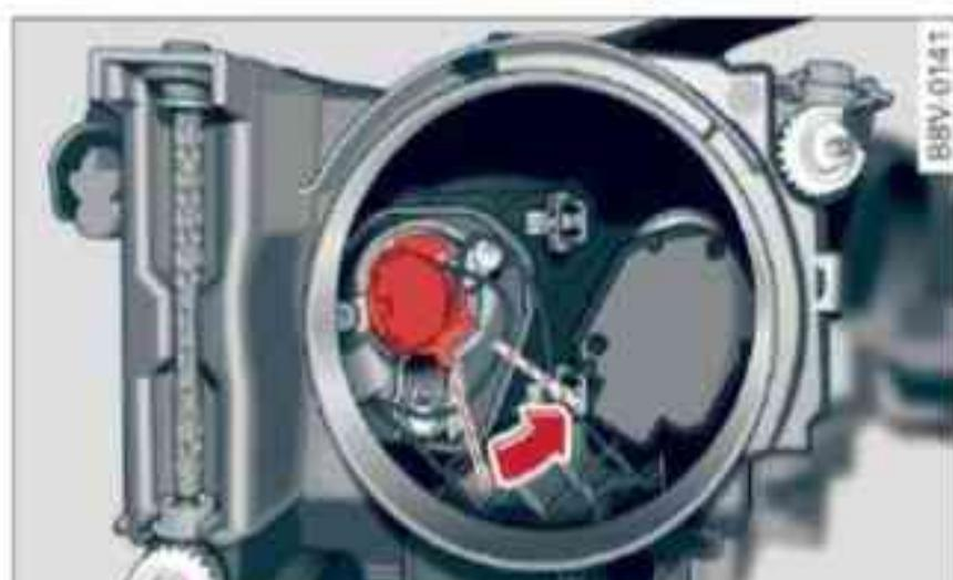
Fig. 269 Bulb housing: Bulb holder for dipped headlights
