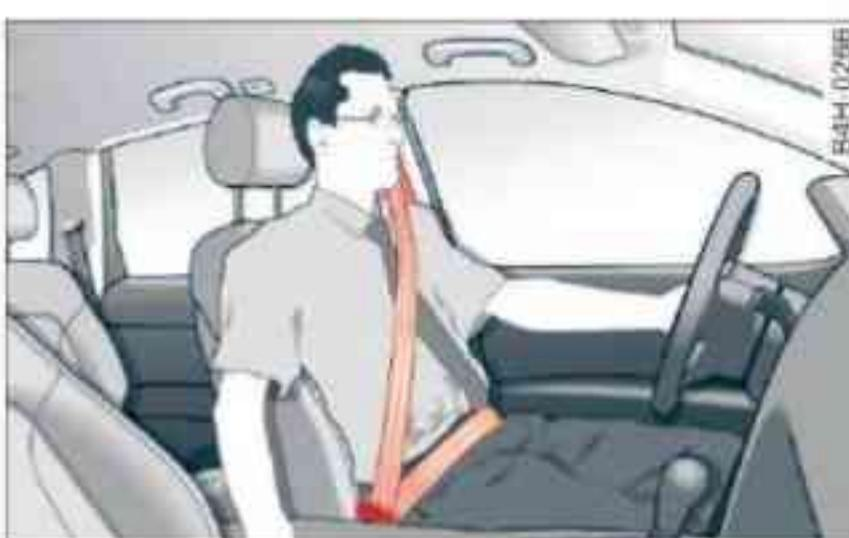
Fig. 181 Positioning of head restraints and seat belts
