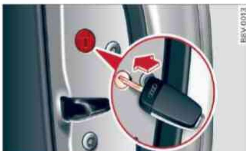
Fig. 41 Locking the door manually
