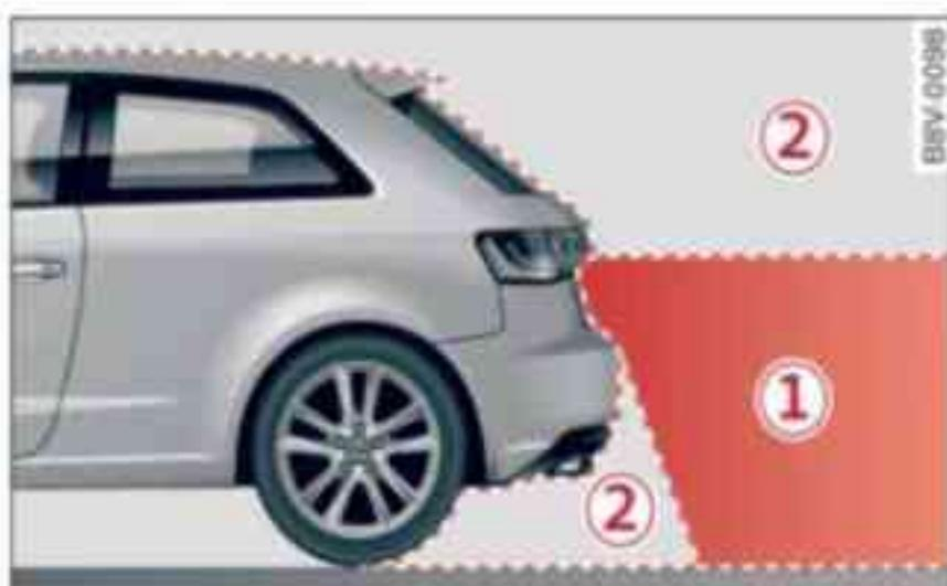
Fig. 152 ①: Area covered by the reversing camera; ②: area NOT covered by the reversing camera (example)
