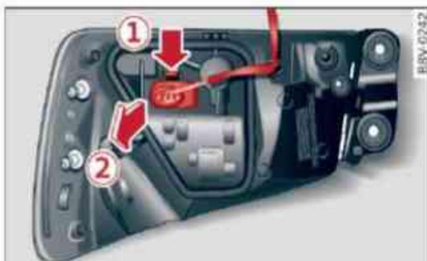
Fig. 309 Rear light: Unplugging connector
