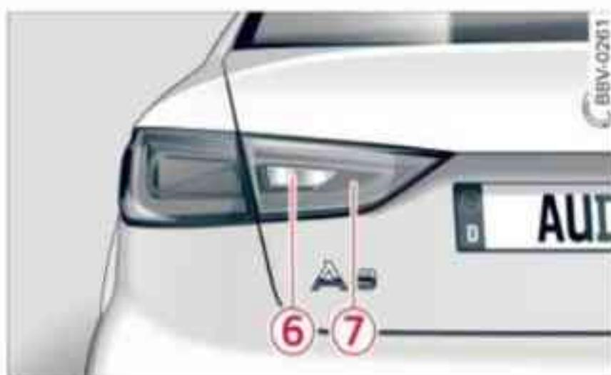
Fig. 267 Xenon/LED system, rear light: Bulbs in side panel and boot lid
