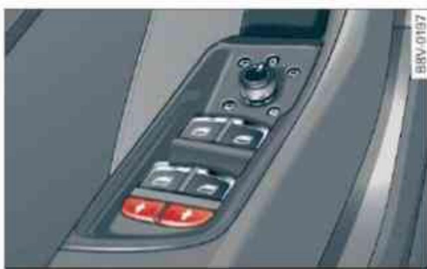
Fig. 47 Detail of driver's door: child safety switches
