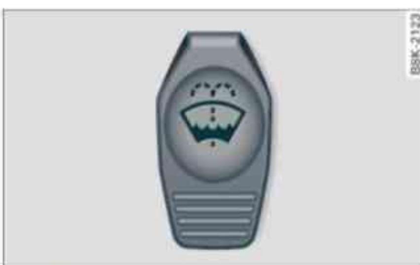
Fig. 226 Engine compartment: Cap of windscreen washer container
