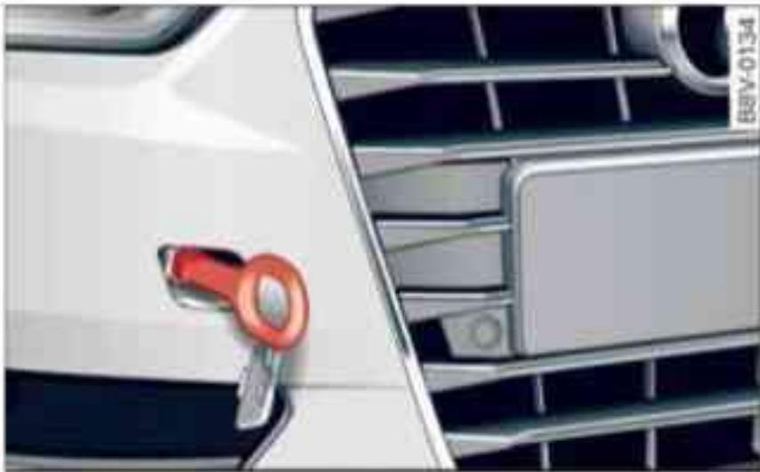
Fig. 252 Front bumper (right side): Towline anchorage screwed in
