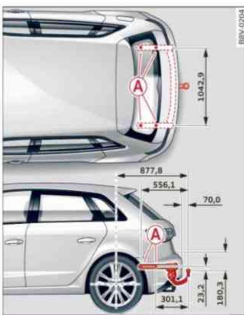
Fig. 213 A3 Sportback: Positions of securing points (viewed from above and from side)
