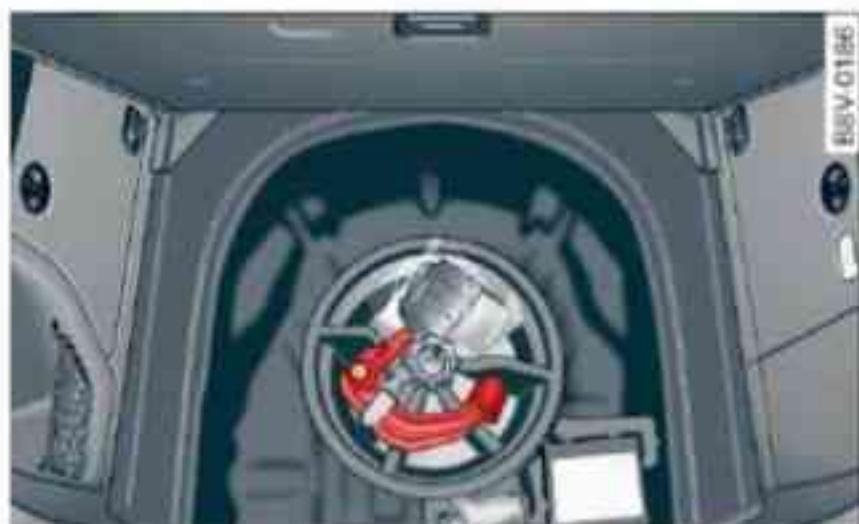
Fig. 202 Luggage compartment: Ball joint for towing bracket (stowage example)
