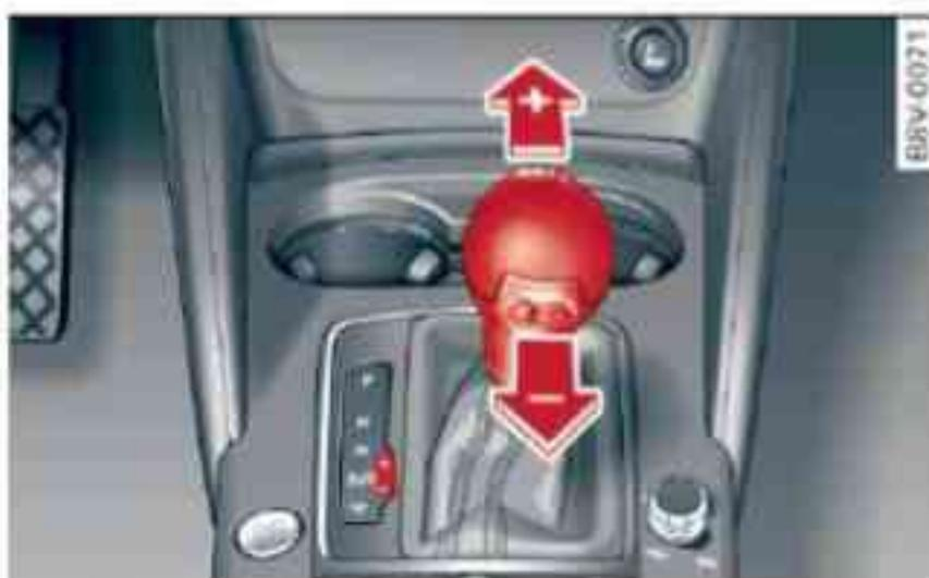
Fig. 120 Centre console: Manual gear selection using selector lever
