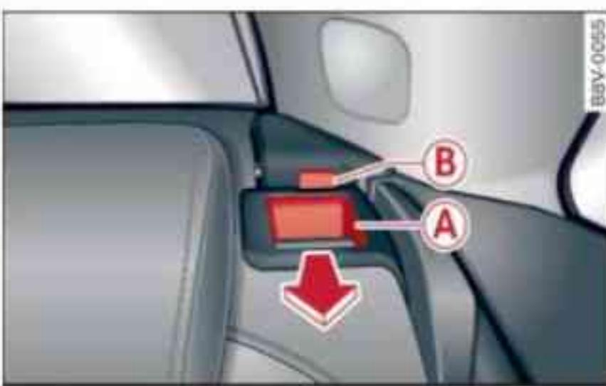
Fig. 85 Backrest: Release lever (example of left side)
