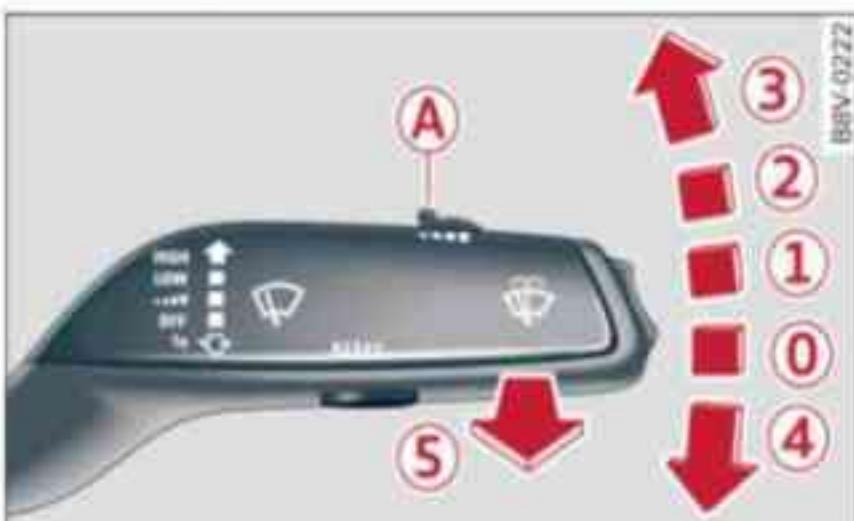
Fig. 62 Windscreen wiper lever: Operating the windscreen wipers (example shows vehicle without rear window wiper)
