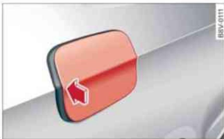
Fig. 115 Vehicle as seen from the rear right: Opening the fuel tank flap
