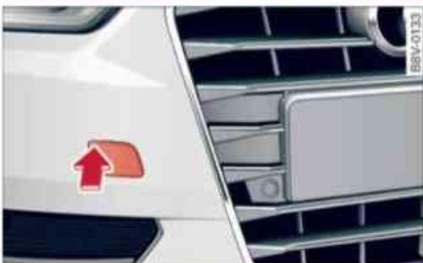
Fig. 251 Front bumper (right side): Removing cover
