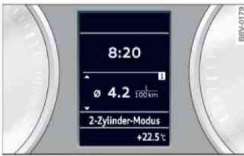
Fig. 23 Instrument cluster: 2-cylinder mode display
