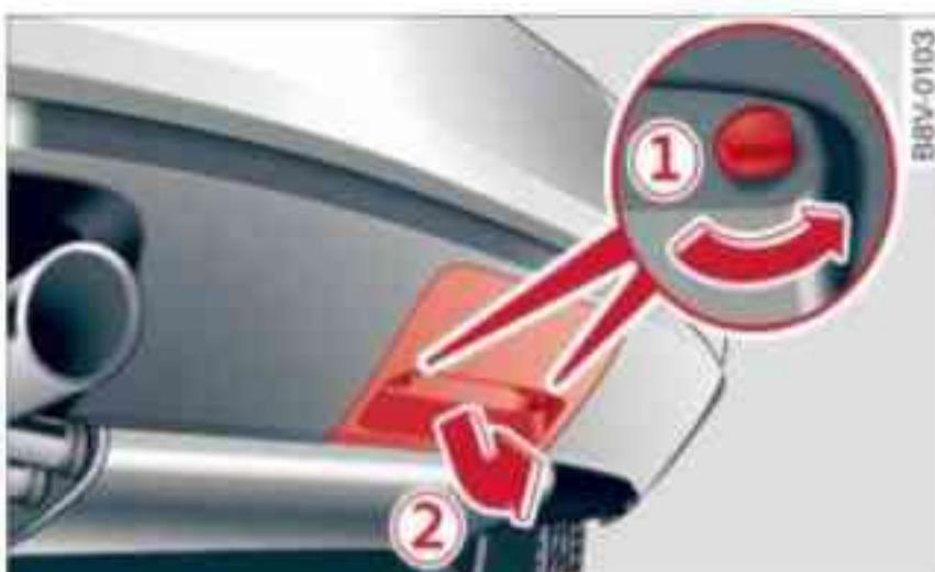
Fig. 203 Area below rear bumper: Removing bumper cover (example)
