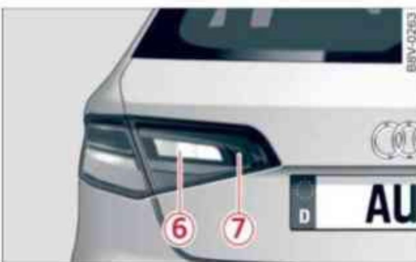
Fig. 265 Xenon/LED system, rear light: Bulbs in side panel and boot lid
