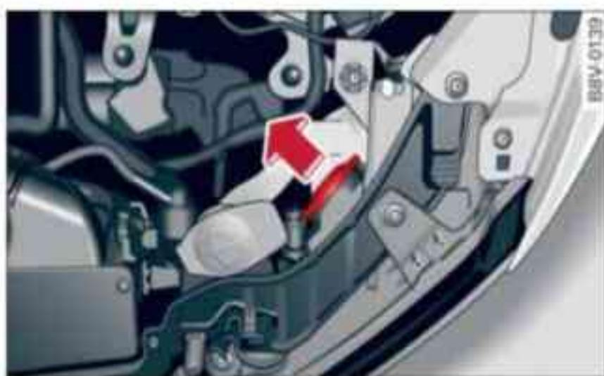
Fig. 275 Engine compartment: Removing cover (side lights)
