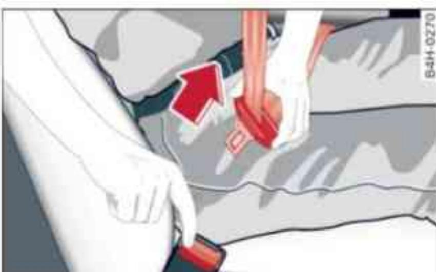
Fig. 186 The latch plate of the belt springs out of the buckle
