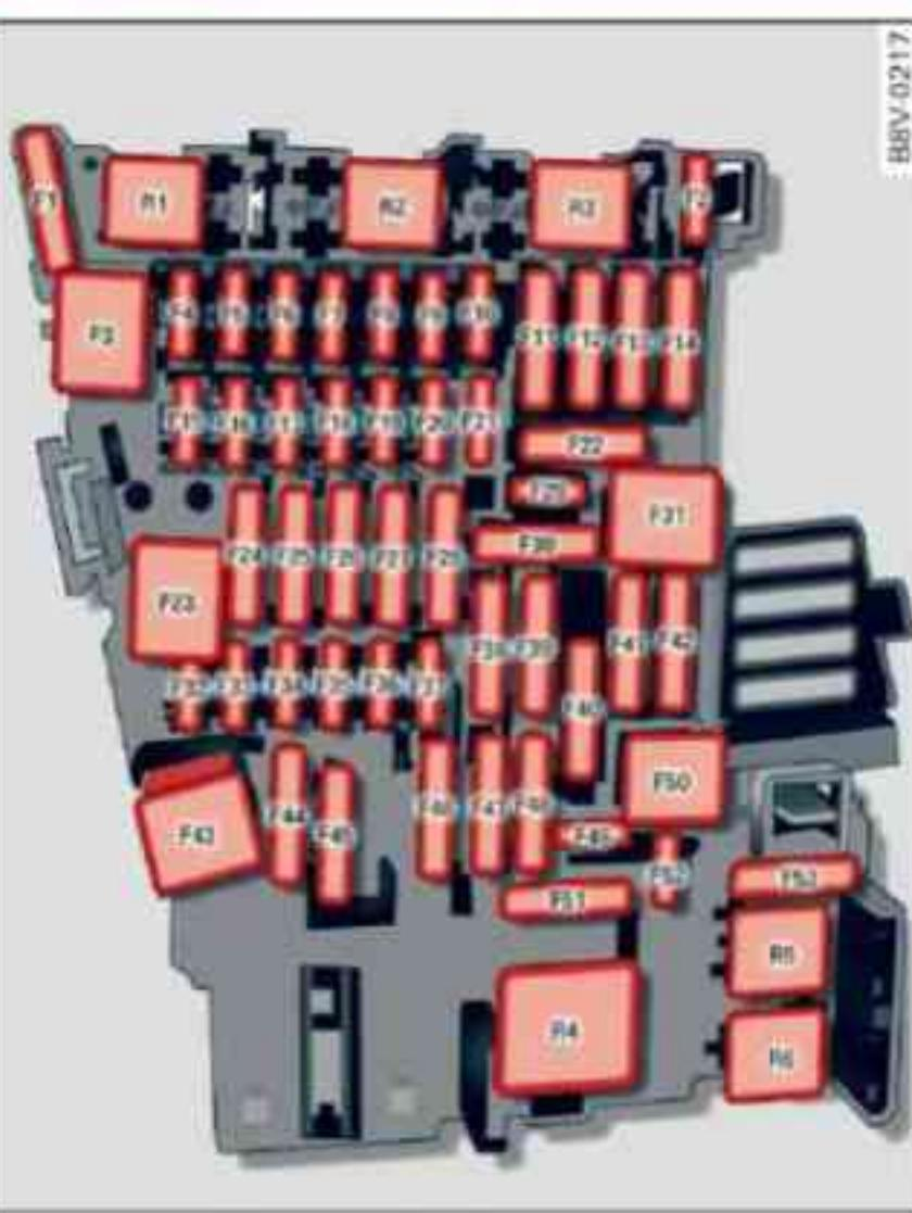
Fig. 258 Interior: Fuse layout
