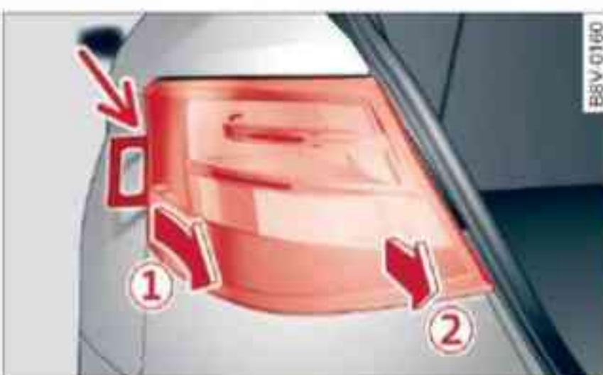
Fig. 292 Removing rear light
