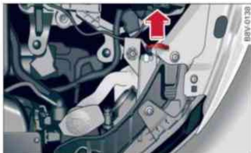
Fig. 268 Engine compartment: Removing cover (dipped headlights)
