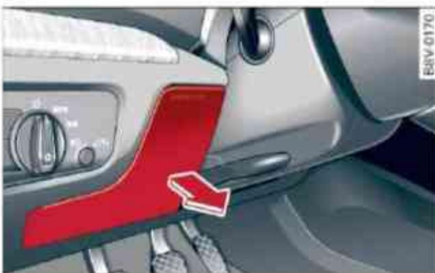
Fig. 255 Area near steering column on LHD vehicle: Cover
