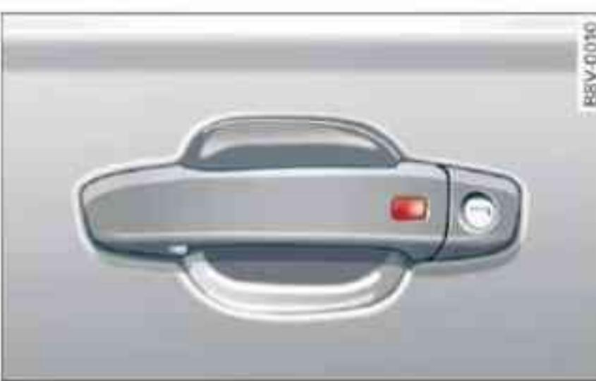
Fig. 38 Driver's door: Locking vehicle with convenience key
