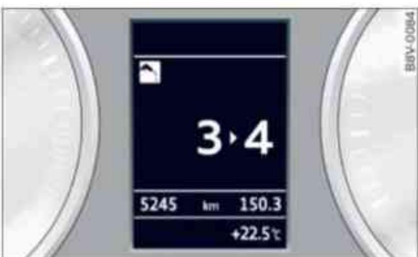
Fig. 19 Instrument cluster: Advanced gear-change indicator on vehicles with monochrome display
