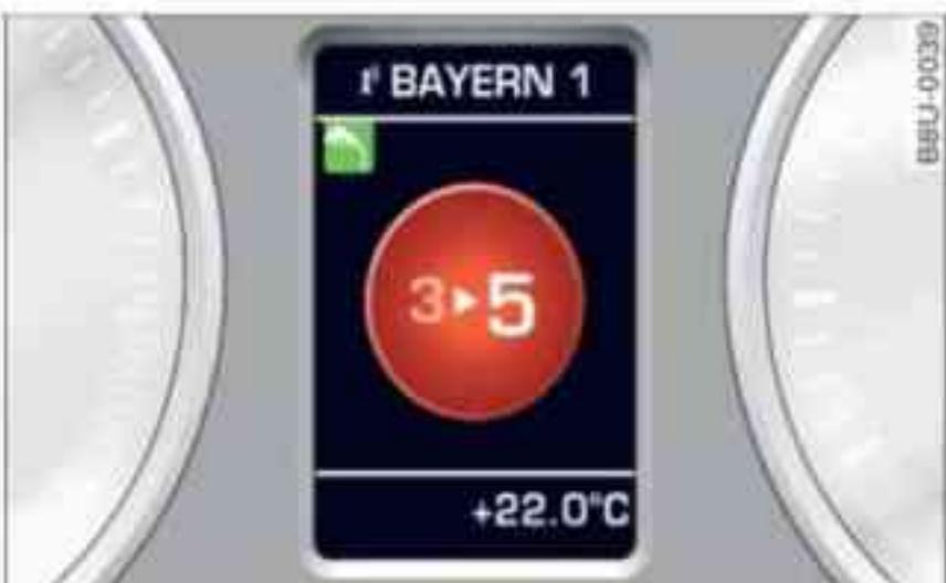
Fig. 20 Instrument cluster: Advanced gear-change indicator on vehicles with colour display
