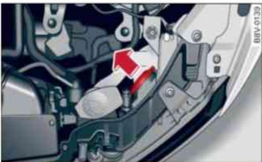
Fig. 272 Engine compartment: Removing cover (main beam headlights/daytime running lights)
