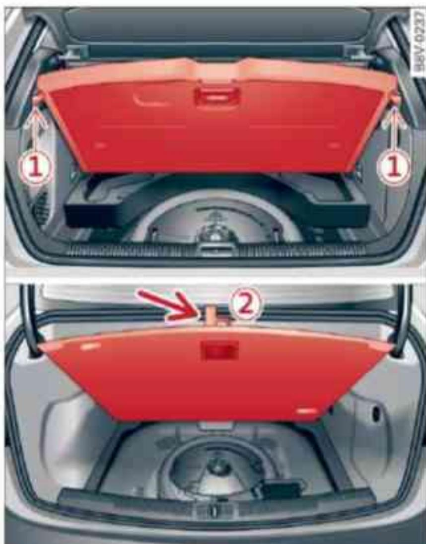
Fig. 247 Luggage compartment: Floor panel folded up (A3 and A3 Sportback top, A3 Saloon bottom)
