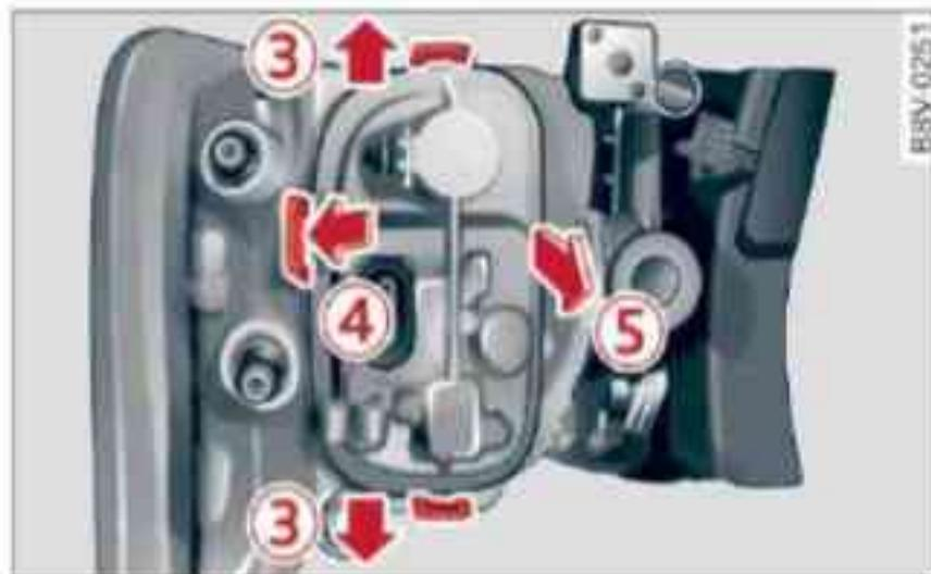
Fig. 296 Securing tabs between bulb carrier and rear light
