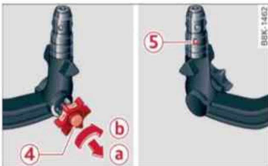
Fig. 206 Removable towing bracket: Setting the spring mechanism to the "ready" position
