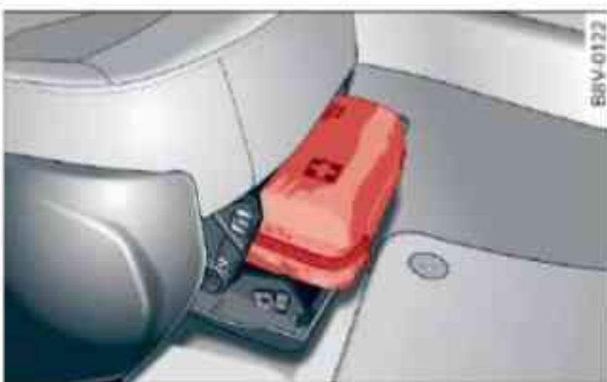
Fig. 234 Right front seat: Stowing the first-aid kit (example)
