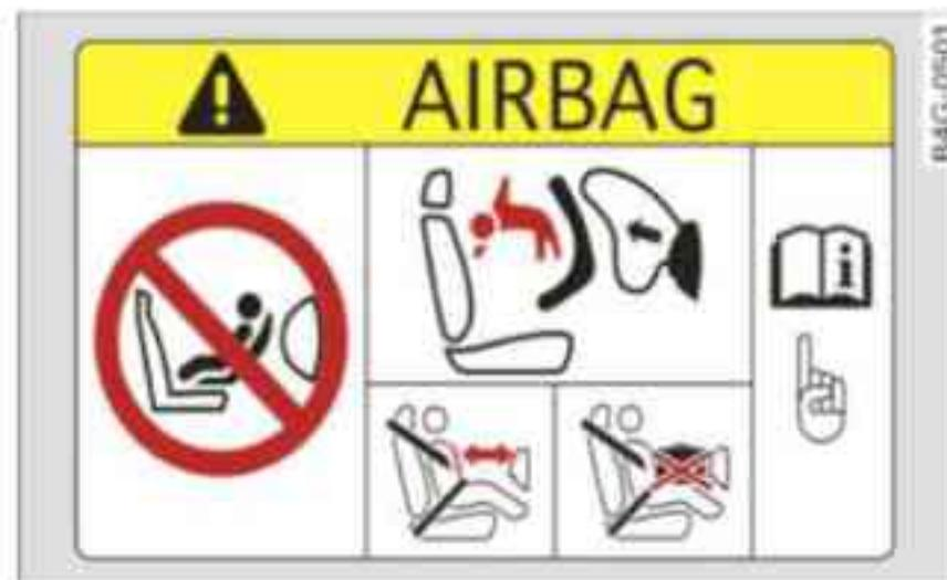
Fig. 187 Front passenger's sun visor: Airbag sticker
