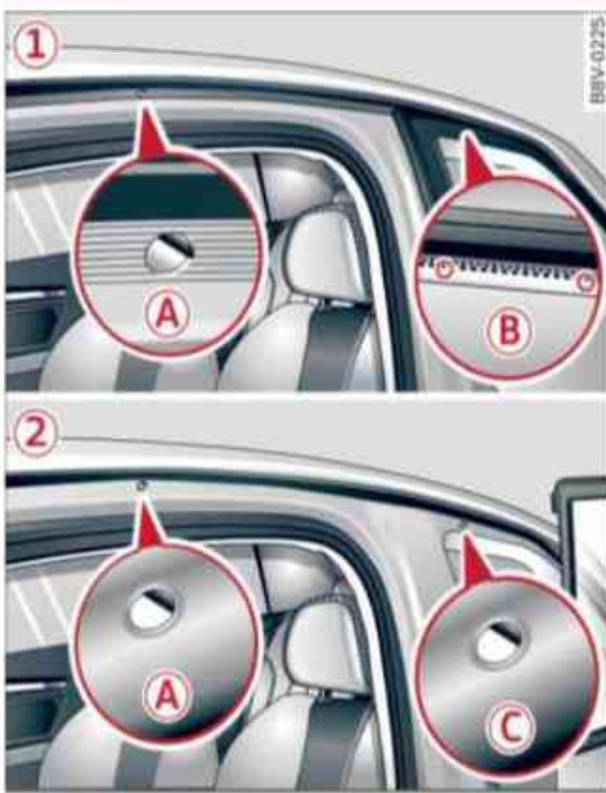
Fig. 82 1) A3, 2) A3 Saloon and A3 Sportback (without roof railings): Attachment points for roof carrier
