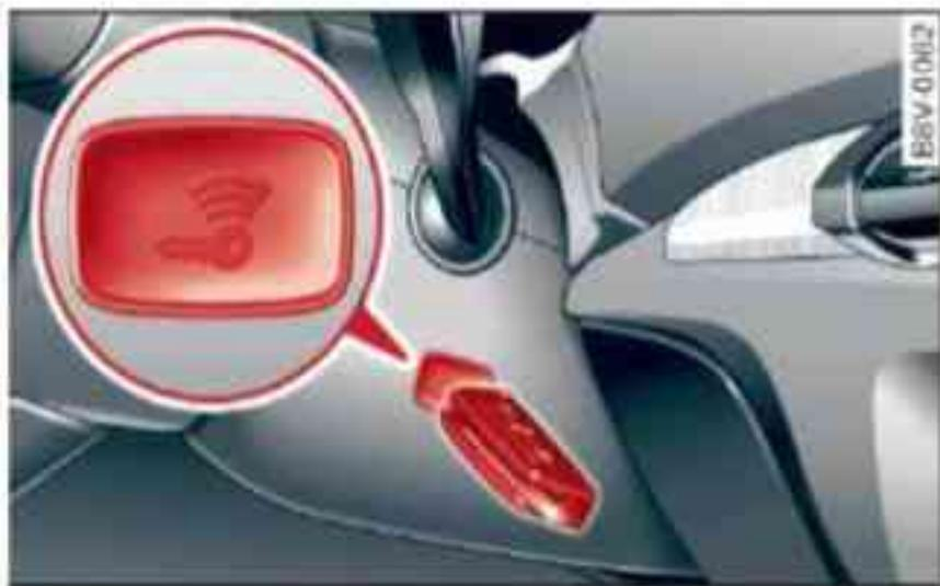
Fig. 105 Steering column/remote control key: Starting the engine after a malfunction
