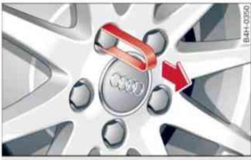
Fig. 240 Wheel: Wheel bolts with caps
