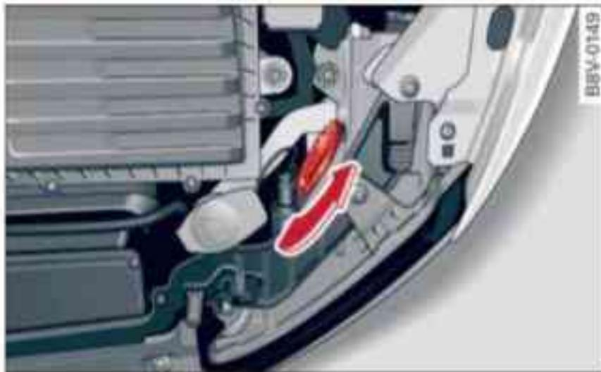
Fig. 281 Engine compartment: Removing cover
