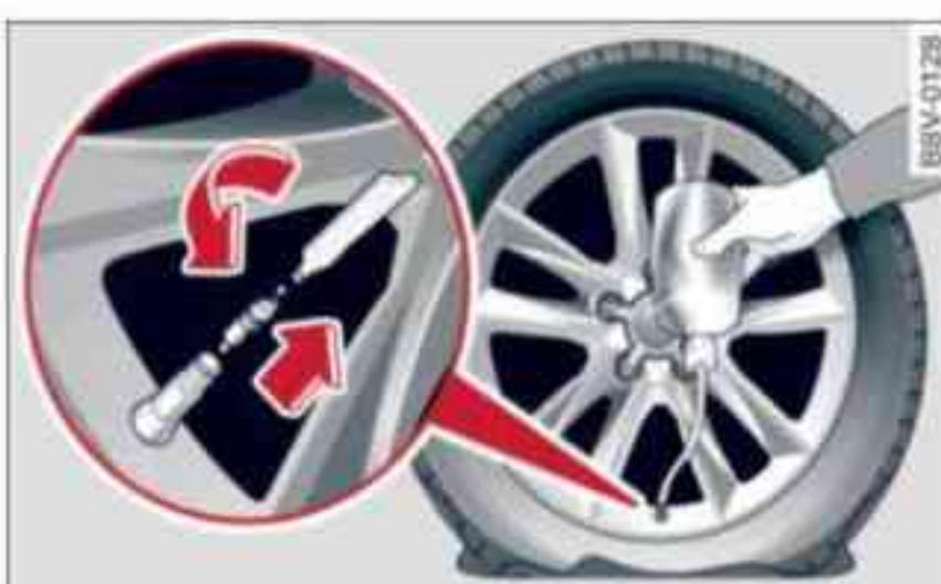
Fig. 238 Tyres: Filling the tyre
