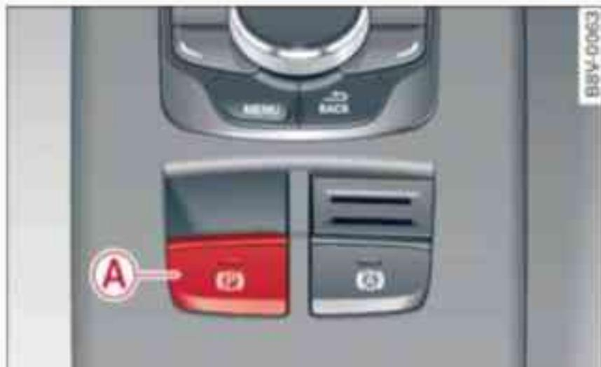
Fig. 106 Centre console: Parking brake
