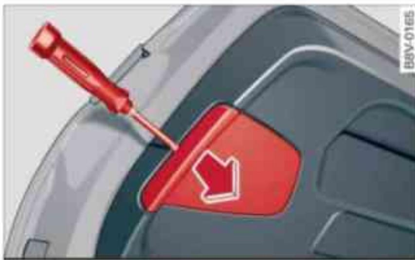
Fig. 301 Open boot lid: Removing cover from boot lid interior trim
