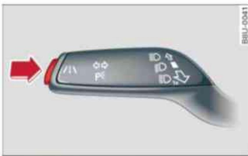
Fig. 137 Turn signal lever: Button for active lane assist
