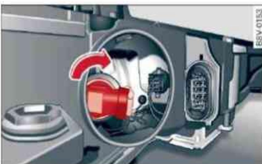
Fig. 286 Bulb housing: Tightening the bulb holder
